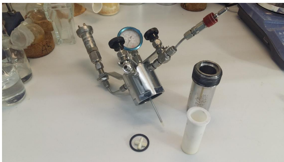
Figure 2.1: Photograph of a stainless steel reactor system used for the coupling reactions involving epoxides and carbon dioxide.
