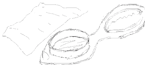
Figure 1-15: Sketch of the cut Eppendorf and the dialysis foil. The sample was added in the cap and then the circle was closed on the cap trapping the dialysis foil in the middle.
