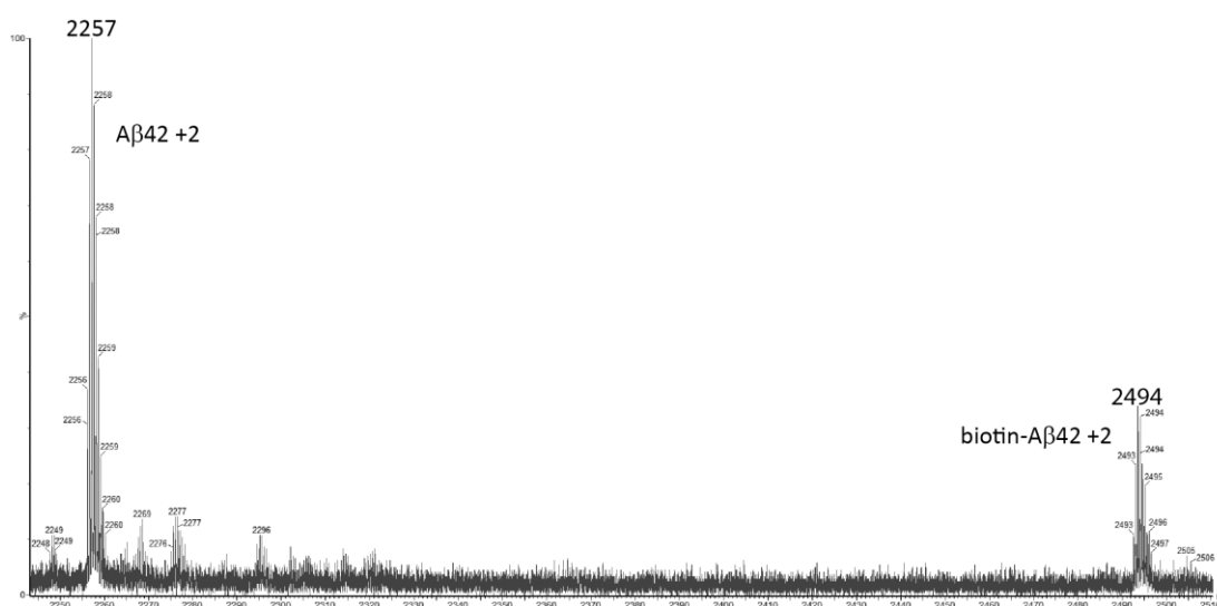
Figure 2-4: MS spectrum of biotinylated \beta PFO. Detection of non-biotinylated monomer with charge +2 at 2257 m/z and biotinylated monomer with a charge +2 at 2494 m/z. The area of the biotinylated peak corresponds to the 25% of the area of both peaks.
