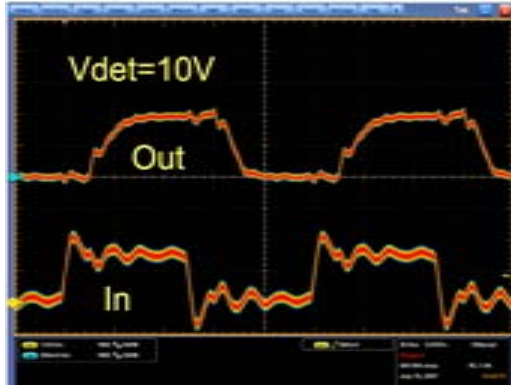
Figure 7.17: Buffer signal, with p+ implantation, detectable for V_{bg} \sim 10V .
