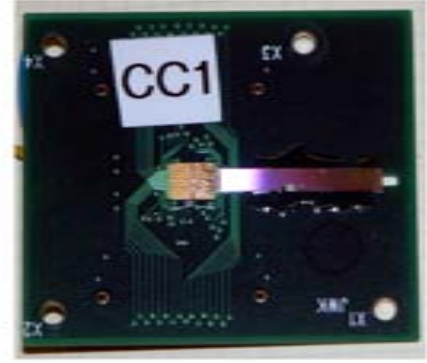
Figure 5.2: CAP3 prototype bonded to a separate board for use with the FE board.
