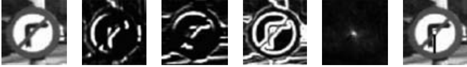
Figure 7.11: (a) Input image, (b) X -derivative, (c) Y -derivative, (d) image gradient, (e) accumulator of orientations, (f) center and radius of the sign.
