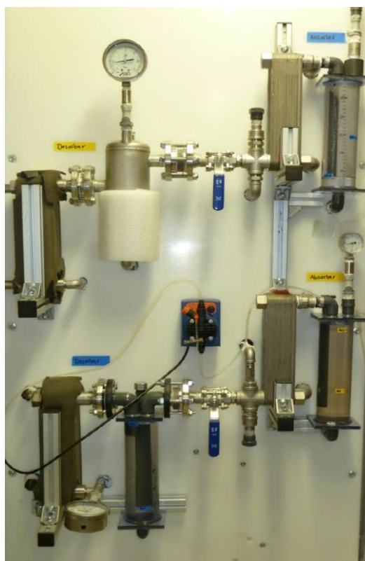
Figure 1.7 1-kW ammonia-water absorption-resorption plant set at TU Dresden [20].
