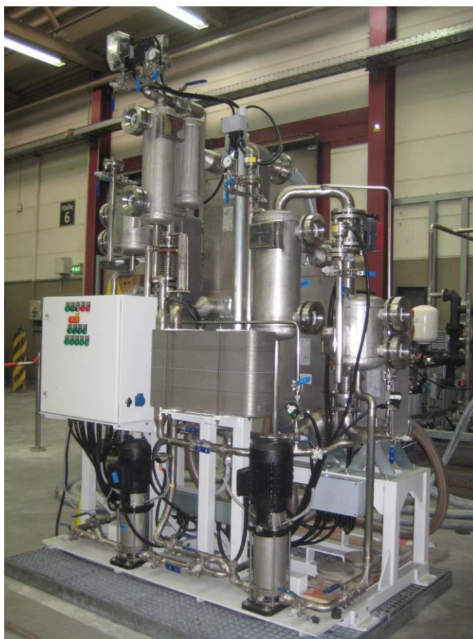
Figure 1.5 80-kW ammonia/water absorption-resorption refrigeration plant delivered by Makatec GmbH to a chicken farm, Geflügelhof Zapf, in Gengenbach (Germany).
