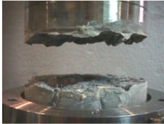
Figure 2.8. Failure at the end
