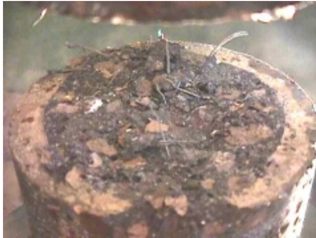
Figure 2.18. Core fracture surface
