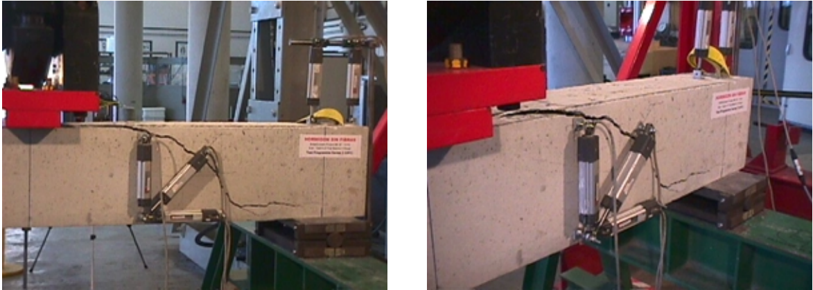
Figure 5.8. Plain concrete 20×30 rectangular beam: Final state of cracking in the critical shear span.
