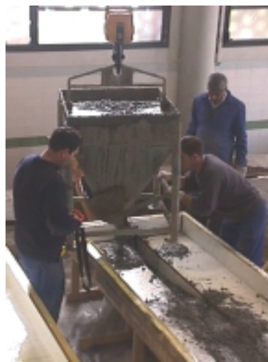
Figure 5.3. Filling of the molds
