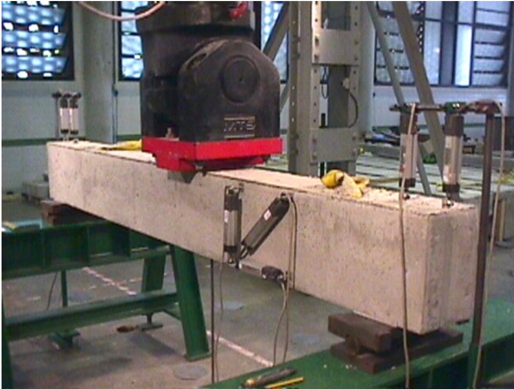
Figure 5.7. Beam ready to be tested
