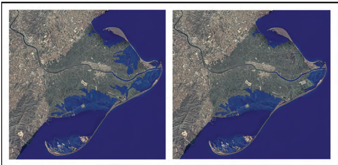
Figure 5.4. Comparison between two possibilities of 33 cm RSLR. The picture in the right exemplify the flood without closing the channels, the left- show what happen if the channels can be closed
