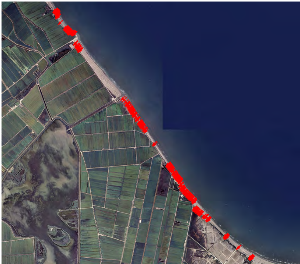
Figure 5.18. Entry points for the overtopping. This points represent places where the high of the beach or the dune is less than the runup, an also for the coastal response could be erode under the runup level.
