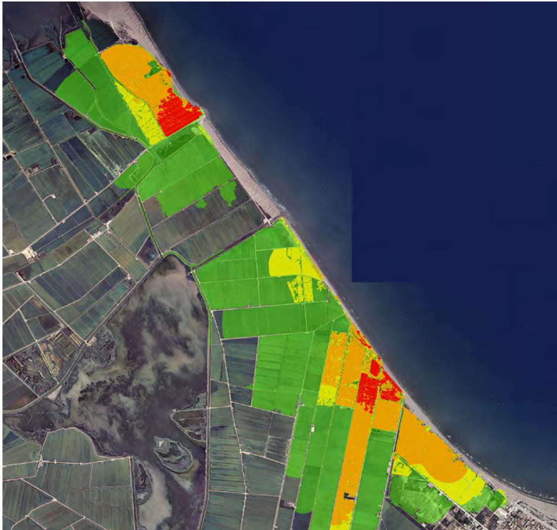
Figure 5.22. Superposition of Potential flood areas, for different return periods. Red color correspond to 10 year, Orange to 50 year, Yellow to 100 year, and Green to 500 years.
