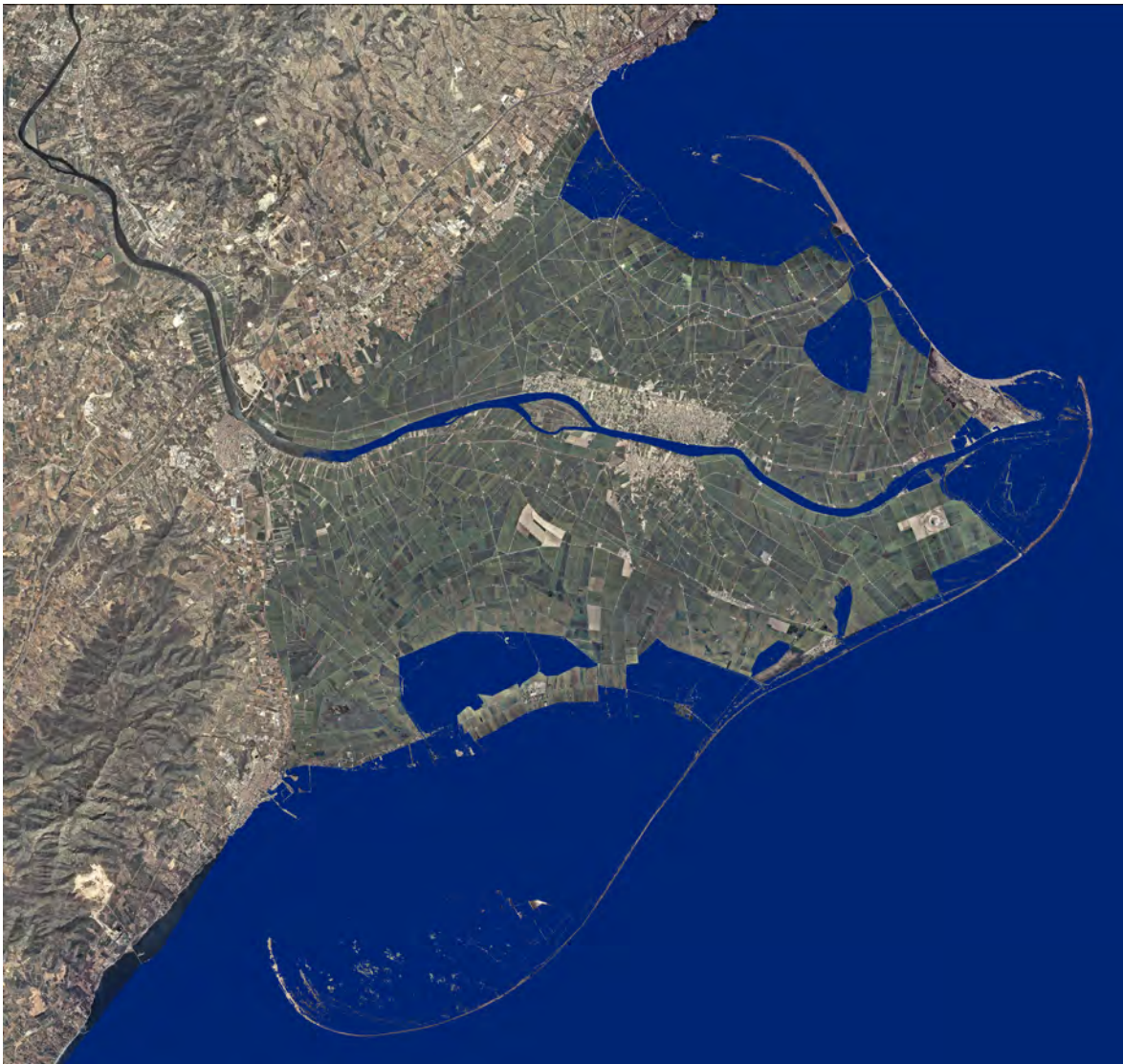
Figure 6.3. Flooded areas in a 55cm RSLR scenario, with the dykes around the contour of the lagoons, and the edge of the delta, as recommended in this work.
