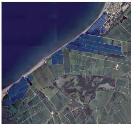
Figure 9. Flood hazard map for 100 years return period storm in the northern part of the Ebro delta (blue areas within the delta).
