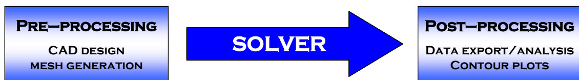
Figure 2.4. Operational structure of commercially-available CFD codes
