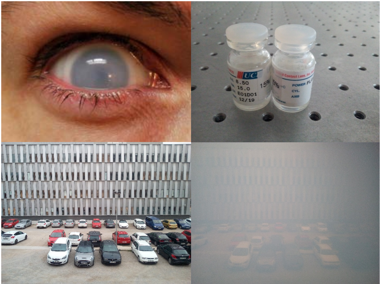
Figure 5.19. Eye wearing the commercial Cataract CL (Image from the vendor website) (top left). Scatter-customized CLs (top right). Images with the same camera without CL (bottom-left) and with a 50% CL attached to the objective lens (bottom right).
