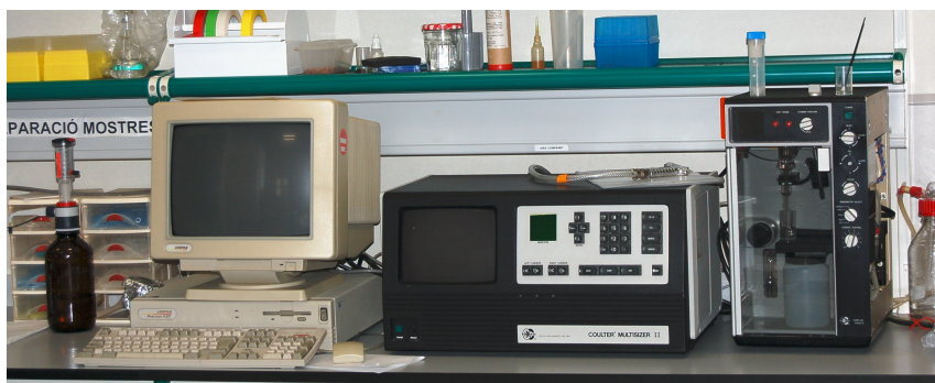
Figure 5.3: Multisizer II electronic particle analyzer (Coulter Corporation ®). Scientific-Technical Services UB (SCT-UB, Serveis Científicotècnics UB).
