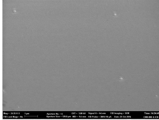
Figure 6.5 SEM image of the surface of a pristine device.
