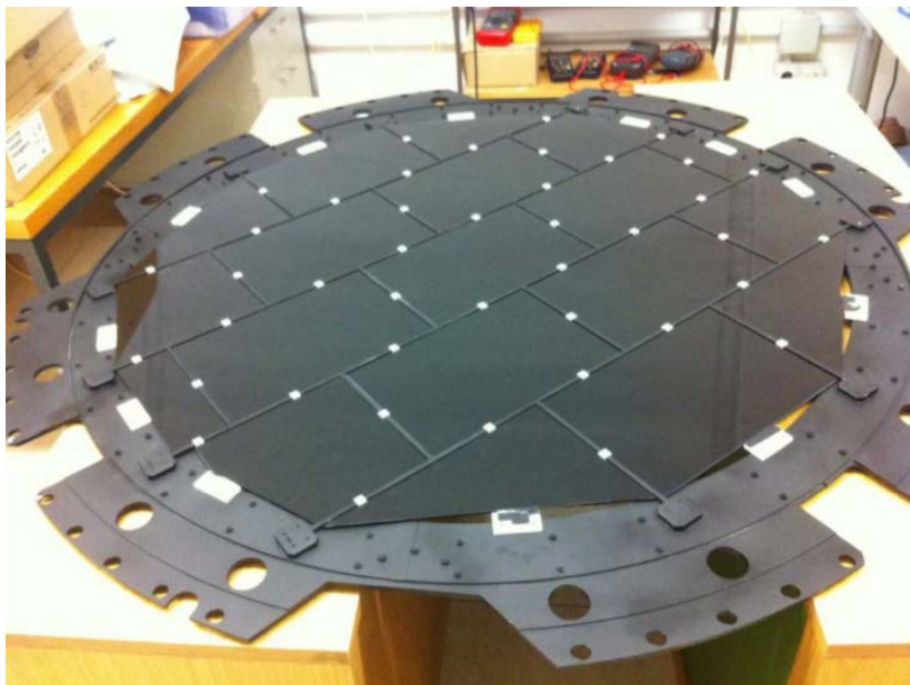
Figure 4.18: Filter frame assembled before mounting in the camera.
