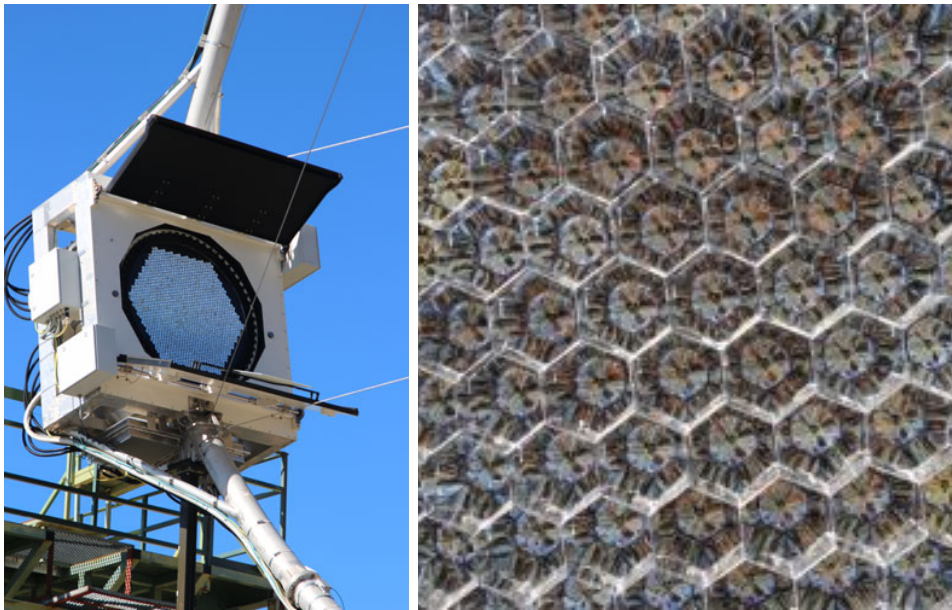
Figure 4.2: Left: One of the MAGIC cameras. Right: PMTs and Winston cones arranged in the camera. Pictures from https://magic.mpp.mpg.de .
