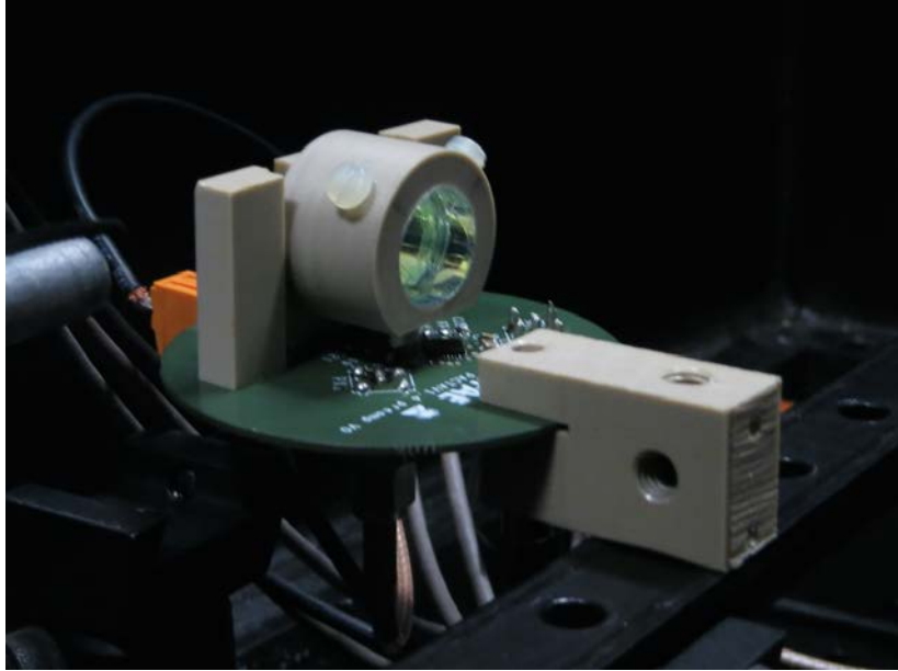
Figure B.15: Image of the Light-Trap holder and electronics board. The SiPM sits on the board upwards in this picture and the disk surface is pointing to the right.
