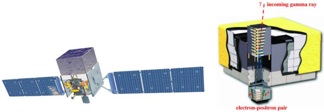
Figure 2.7: Left: The Fermi Gamma-ray Space Telescope. Right: The converter/tracker, calorimeter and anticoincidence shield in the LAT detector. Image Credit: LAT collaboration
