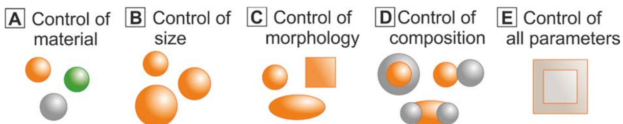
Figure 1.2. Parameter of control for the synthesis of metal NPs. Adapted from reference [4]
