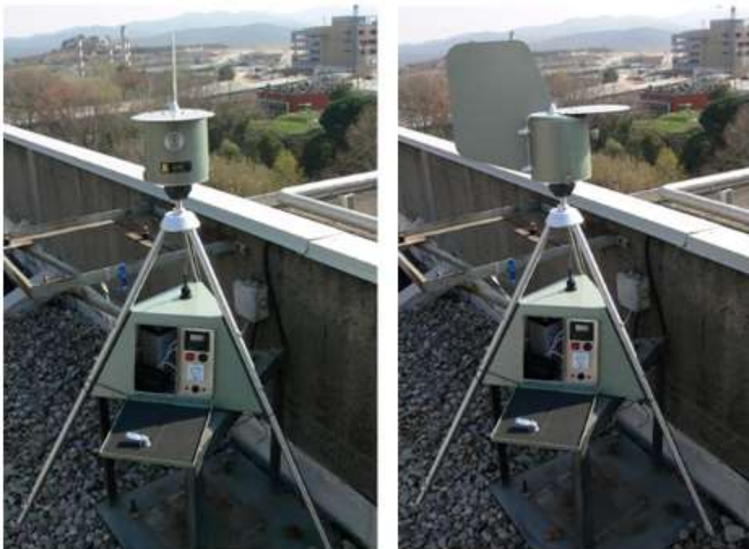
Figure 11. Burkard Multi-vial cyclone air sampler at the C Building of the Universitat Autònoma de Barcelona, in Bellaterra.
