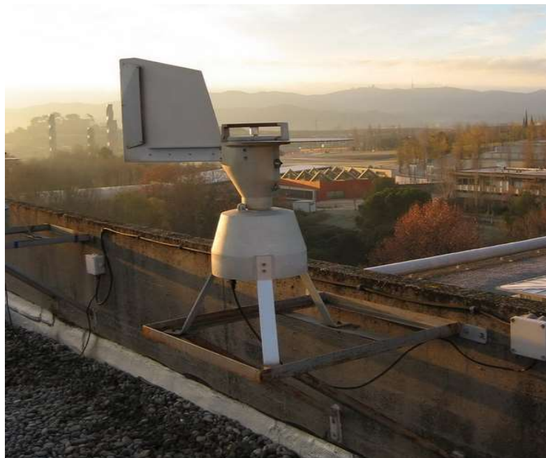
Figure 9. Lanzoni VPP2000 air sampler at the C Building of the Universitat Autònoma de Barcelona, in Bellaterra.
