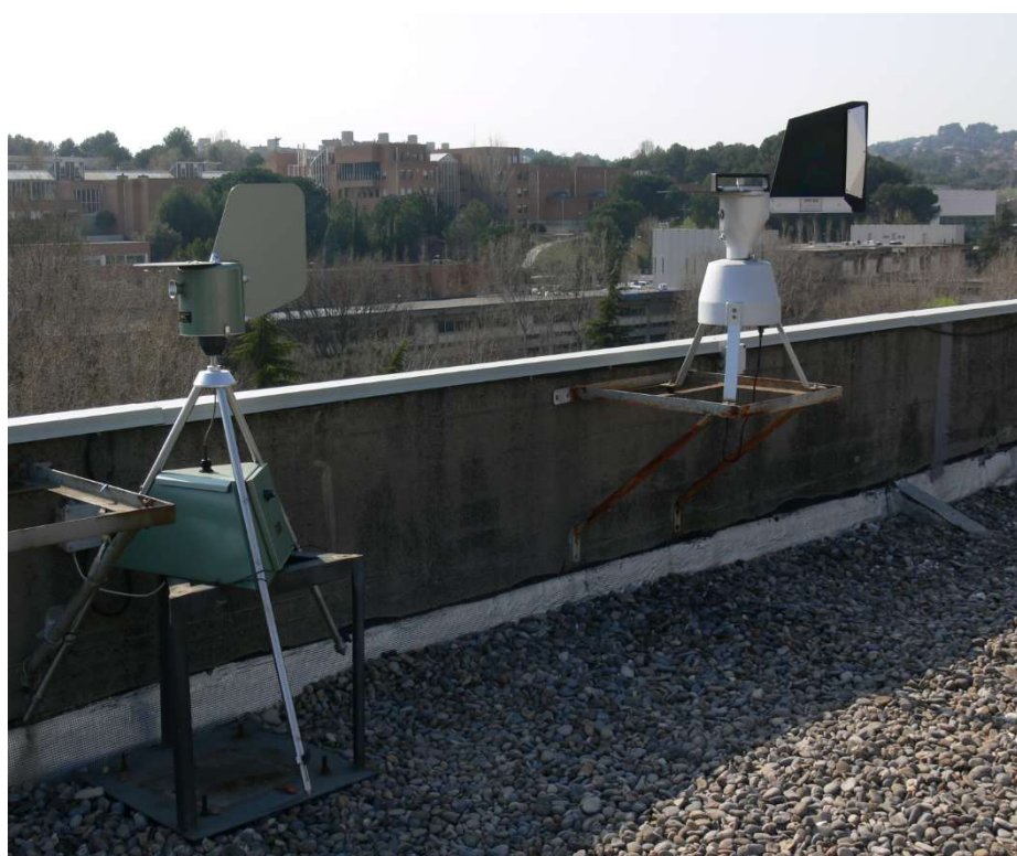
Figure 10. Burkard Multi-vial Cyclone (in front) and Lanzoni VPP2000 air samplers at the C Building of the Universitat Autònoma de Barcelona, in Bellaterra.
