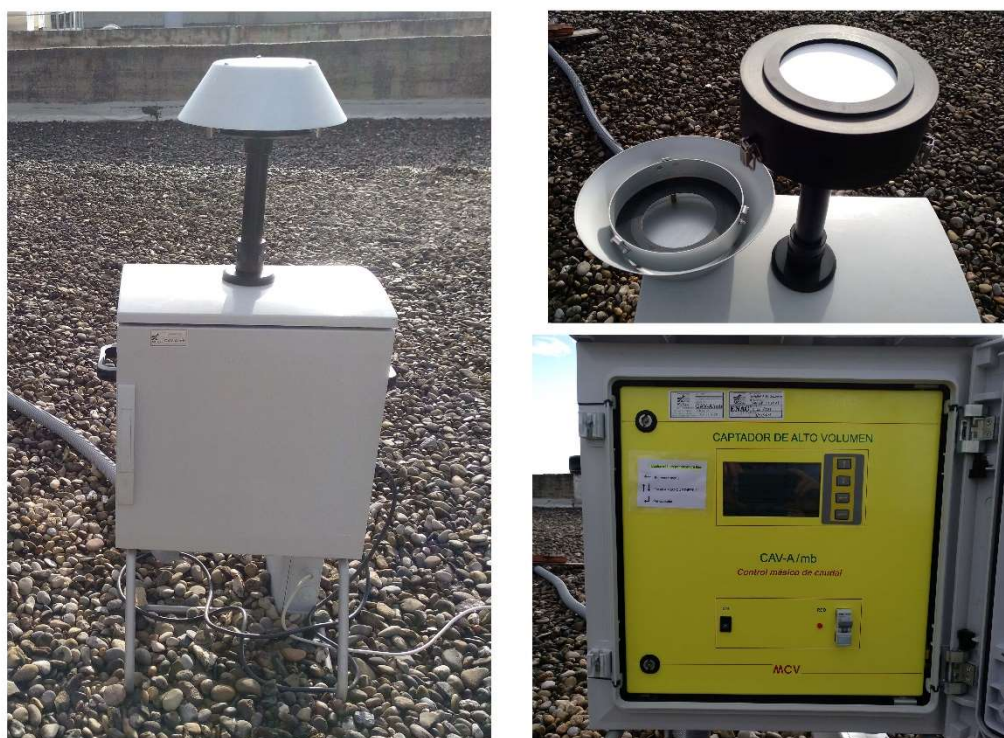
Figure 12. MCV high-volume air sampler at the C Building of the Universitat Autònoma de Barcelona, Bellaterra.
