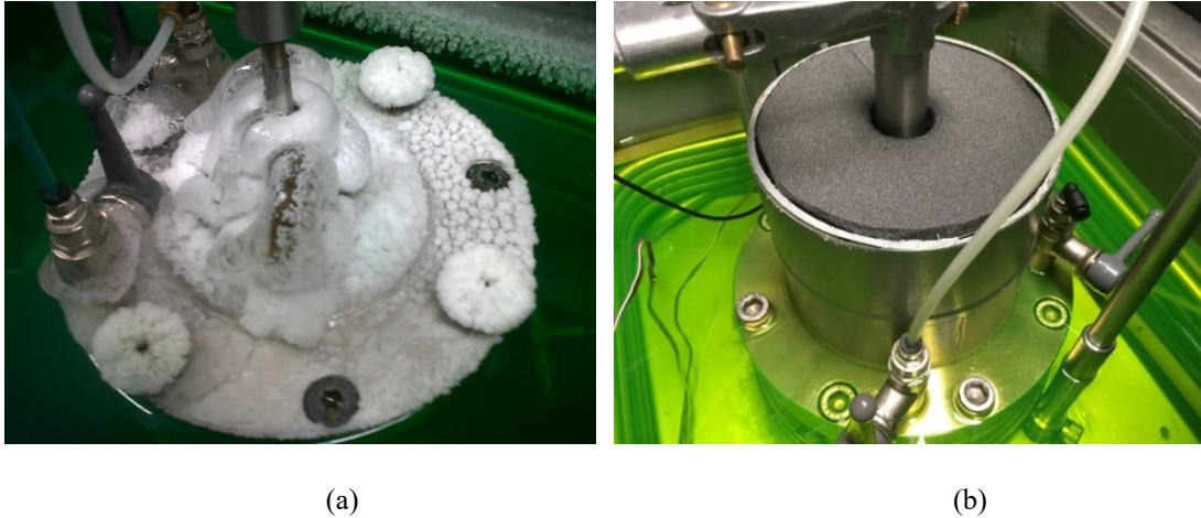
Figure 3.34 Freezing state situation: (a) without insulation and (b) with PVC insulation
