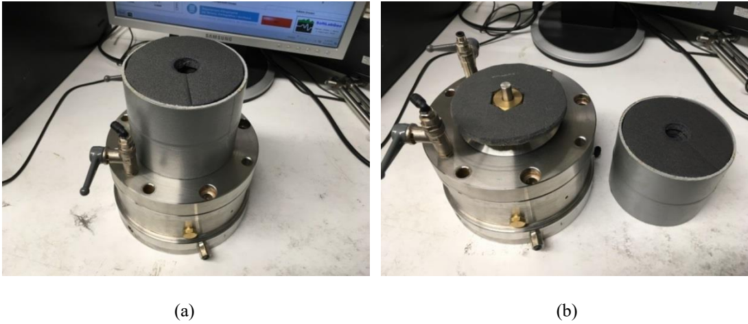
Figure 3.33 Insulation contact area of the piston-rod LVDT with section PVC and polyethylene lining
