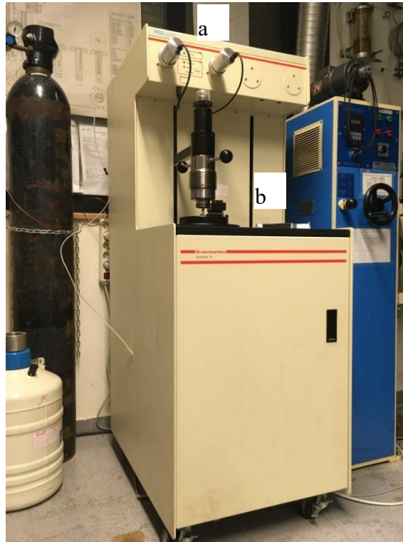
Figure 3.39 Mercury porosimeter (AutoPore IV 9500): (a) low pressure ports and (b) high pressure port
