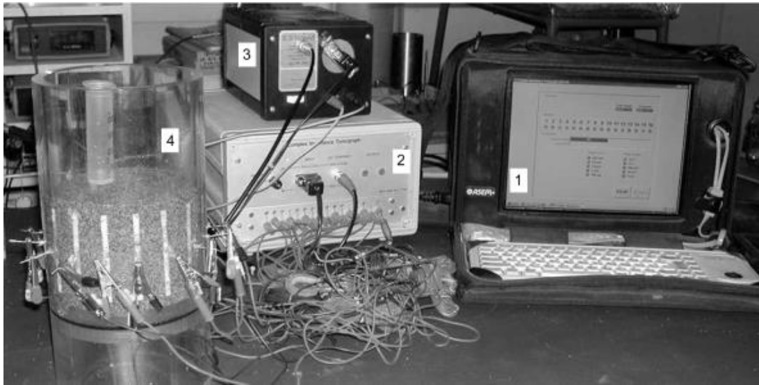
Figure 3.22 Measurement set-up: (1) personal computer; (2) data acquisition system; (3) inverter and (4) measuring cell (Borsic et al., 2005)
