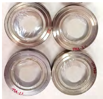
Fig. 4. Holder containing the fresh pastes, sandwiched between thin polyester films, for Cu K \alpha laboratory XRD data collection
