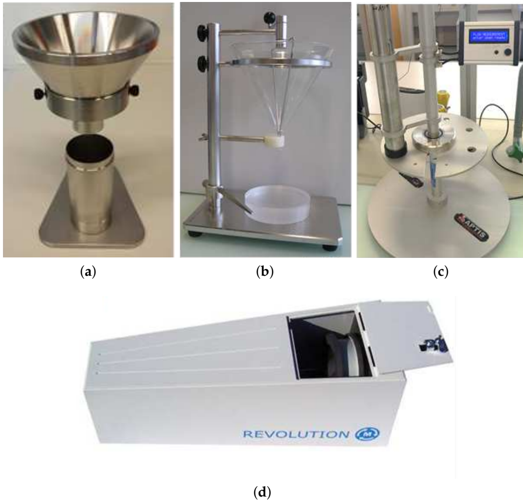
Figure 7.1: Flowability methods used in this study. Free-flow density cylinder (a), Angle of repose apparatus (b), GranuFall (c) and Revolution powder analyzer (d). Courtesy of Nestlé
