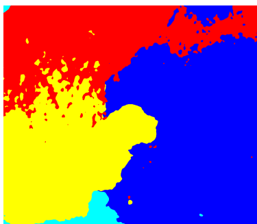
Fig. 3. Unsupervised segmentation of the first orthophoto using Gabor filters with two and four classes.
