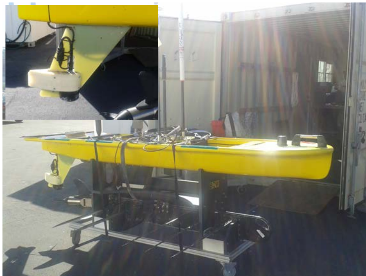
Figure 3.4: The Wave Glider used during the tests, and a zoom of the DAT system installed in the keel (inset)
