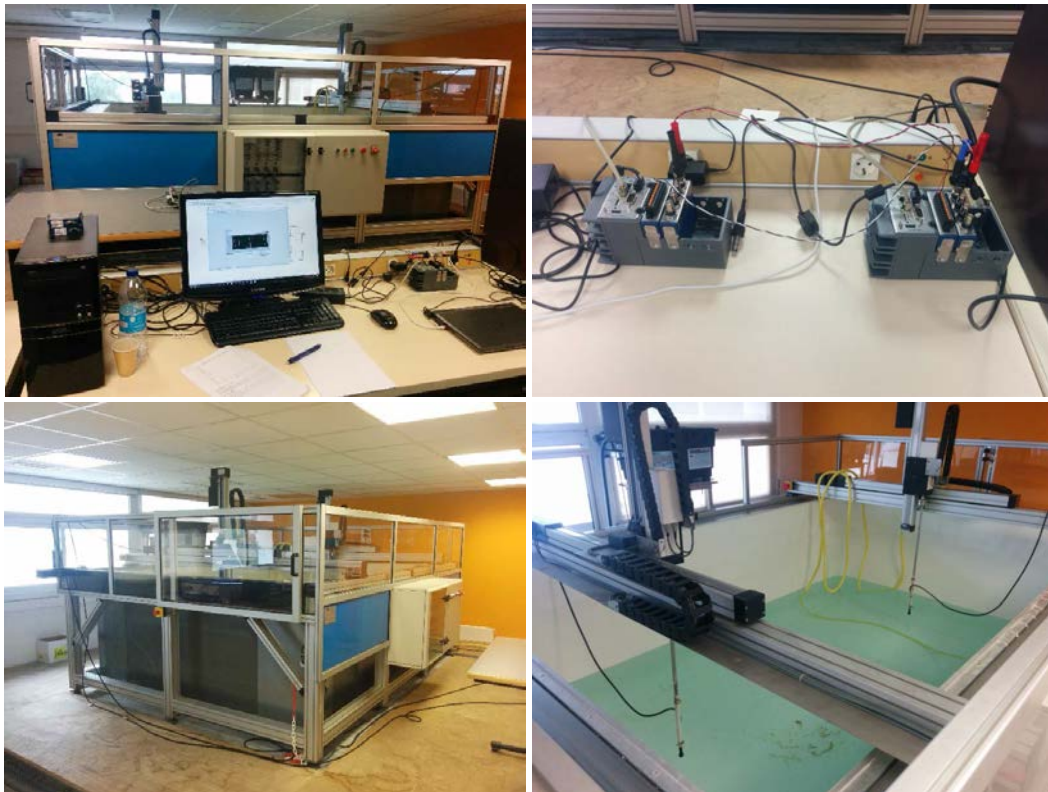
Figure 7.8: Images taken during a laboratory experiment, where the test-tank used and the cRIO modules can be observed.
