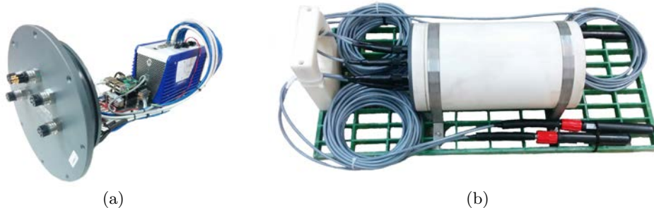
Figure 2.2: The NeXOS A2 system, (a) internal, and (b) external with the A1 hydrophones installed.
