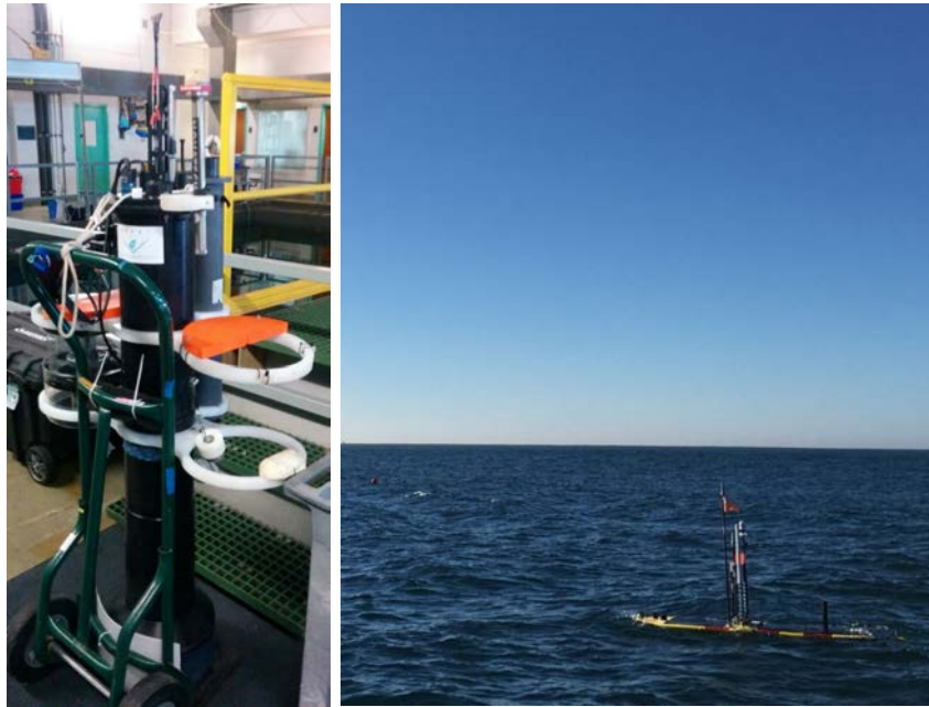
Figure 5.9: Coastal Profile Float (left) and Wave Glider (right) during sea tests conducted at Monterey Bay, California.
