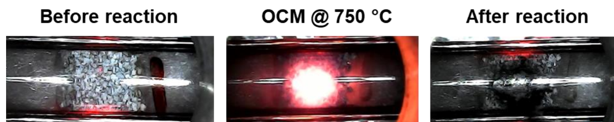
Figure 5.7 Pictures of La_2O_3 -SiC catalyst bed before OCM reaction (left), during OCM reaction at 750 °C (middle), and after OCM reaction (right). The gas flow is from the left to the right of the reactor tube.
