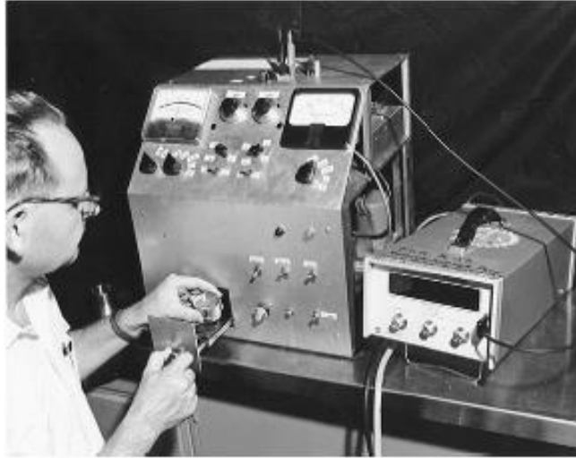
Figure 2. Reproduction of picture of the first NIR instrument developed by Norris et al. for moisture measurement of wheat flour. Taken from reference [10] (doi:10.1016/j.trac.2010.01.003).
