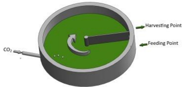
Figure 1.2. Circular open pond used in biodiesel production processes (Kiran et al., 2014)
