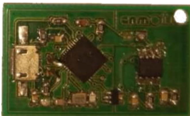
Figure 5.6. Picture of the potentiostat fabricated in collaboration with ICAS group of IMB-CNM. 170
