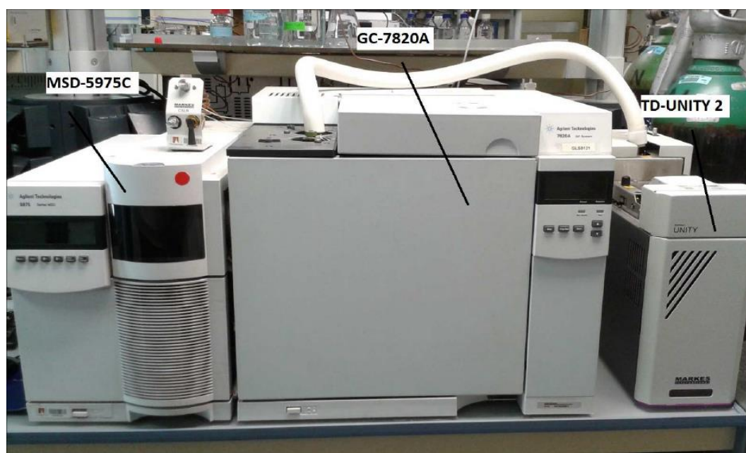
Figure 4.3. TD-GC/MS system used for VOCs characterization.
