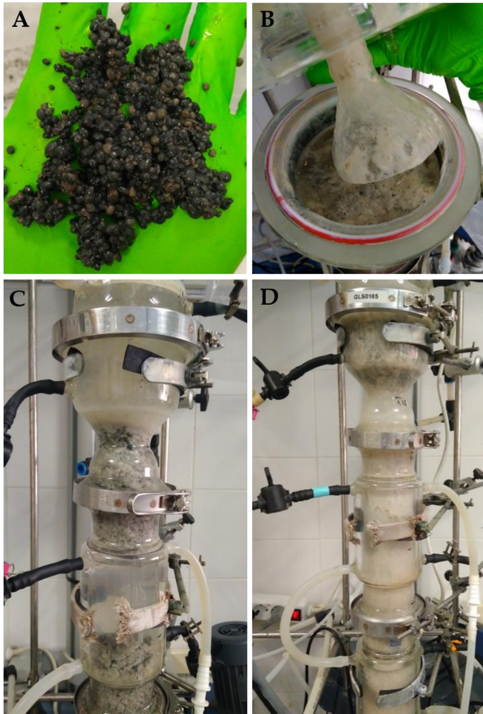
Figure 7.1. UASB described in Chapter 5. A) Granular sludge (inoculum); B) Slime attached to the upper part of the reactor (day 490); C) Day 300 of the operation; D) Day and 400 of the operation.
