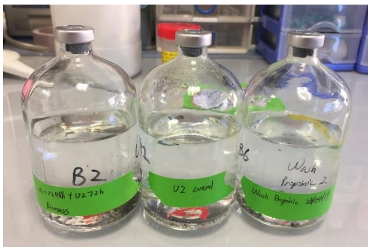
Figure 8.1. Bottles with granular biomass used for the enrichment test. Two bottles were used as experimental ones (fed with sulfate) and the other one was the control bottle (fed without sulfate).
