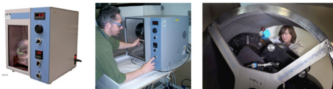
Figure 1.2 CCC devices commercialized by Dynamic Extractions (Slough, UK). a) MiniCCC, internal volume 18 mL, processed samples 10-300 mg; b) MidiCCC, internal volume 19-940 mL, processed samples 15-25 g with the bigger column; c) MaxiCCC, internal volume 18,000 mL; processed samples 1,500 g.
