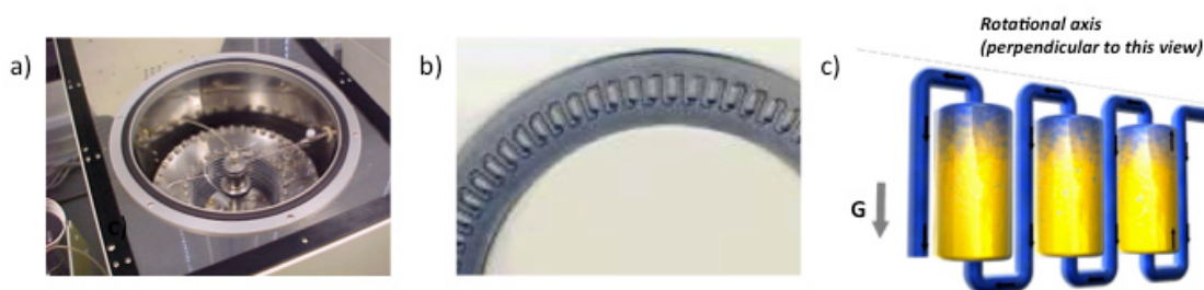
Figure 1.3 Hydrostatic CCC column. a) Detail of the rotor of a CPC column. The rotor has a single vertical rotating axis. b) Image of one of these disks. c) Schematic representation of the ducts and channels engraved in the disks that constitute the rotor. In this case the denser phase (yellow) acts as stationary phase while the less dense (blue) is the mobile phase.
