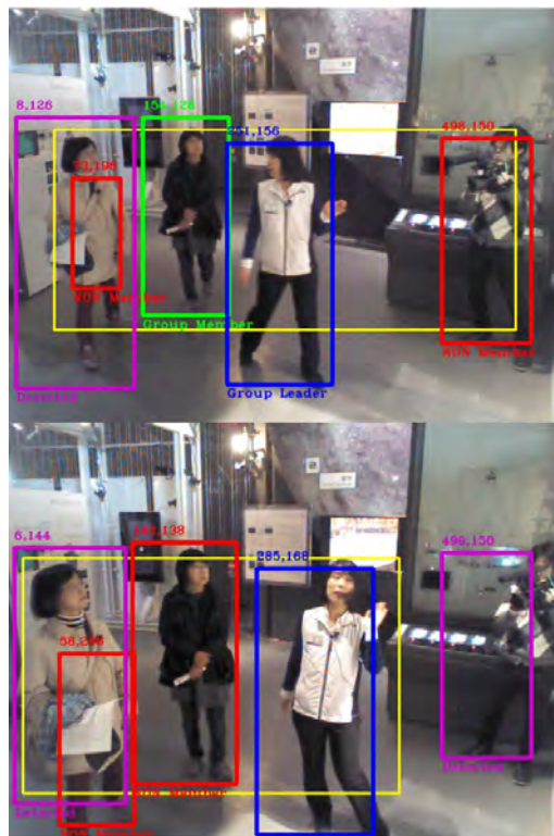
FIGURE 4.17: Video 3 results from exponential motion implementation. Top: Frame 51, even though the four people on the scene are moving as much as the group leader does, the leader is correctly categorized along with the cameraman and one of the two group members. Bottom: Frame 102, two out of three detections are wrongly categorized. Purple boxes reference to previous detections.
