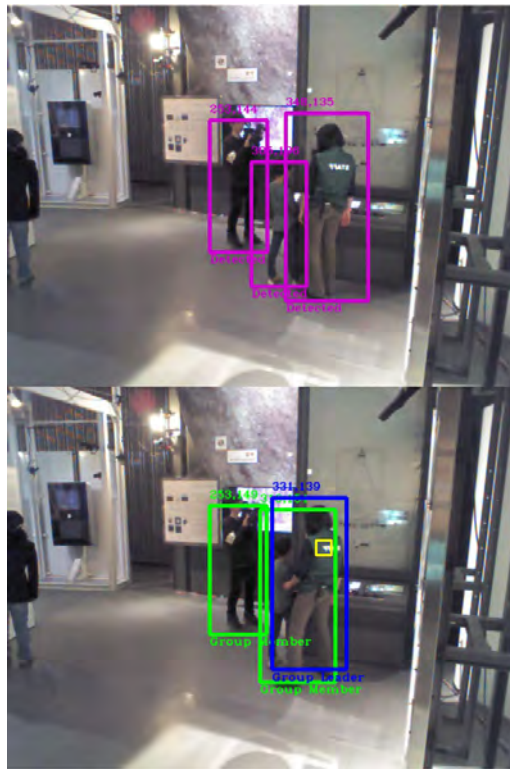
FIGURE 4.6: Training3 video exemplifying a Soft case. Top: Frame 1, people detector outputs three humans on scene. Bottom: Frame 35, the algorithm is able to rapidly categorize all detections after the group leader has been identified.
