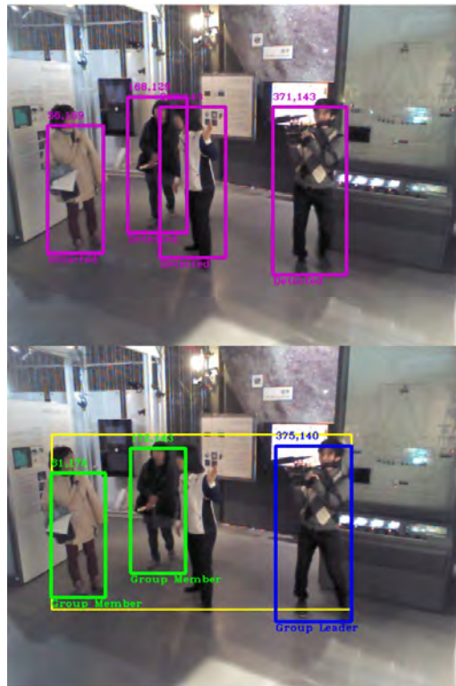
FIGURE 4.14: Video 3 with 46% of accuracy. Top: All individuals are detected, no roles assigned yet. Bottom: Cameraman has been addressed as the group leader, whereas the science communicator is not even detected on this frame. A large motion rectangle is displayed containing all the detections on scene.
