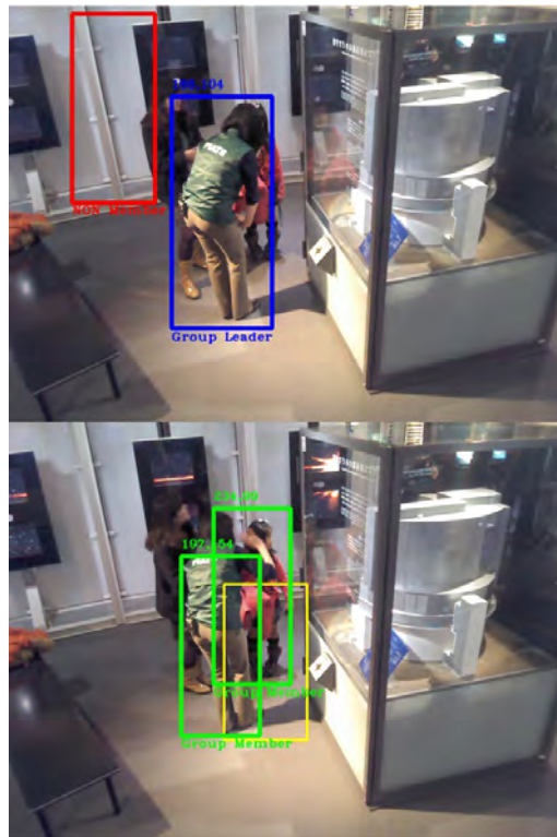
FIGURE 4.13: Video 6 with 70% of accuracy. Top: Science communicator is being tracked as the leader. False positive object detection is classified as non-group member until the algorithm is able to eliminate it. Bottom: Leader tracking is lost in some point around frame 35. Yet, the algorithm still considers the leader as part of the group.
