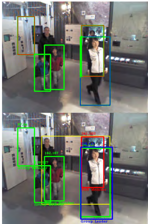
FIGURE 4.8: Sample frame 38 of Video 2. Top: Ground truth annotation. Bottom: Testing result. A blue box represents the Group Leader, green boxes are for Group Members and red boxes suggest Non-Group Members. A yellow box describes the motion detection area, which is rather large on this scene undergoing a Transitory state.
