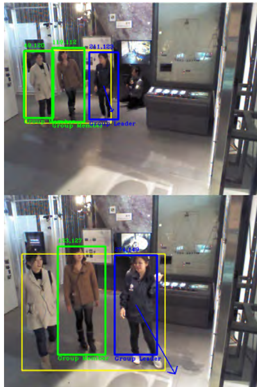
FIGURE 4.10: Video 5 with 98% of accuracy. Top: Sample frame 5. A blue arrow with the leader's torso as origin estimates her direction. Bottom: Sample frame 15. Leader's direction arrow indicates the direction of movement and also displays its proportional magnitude.
