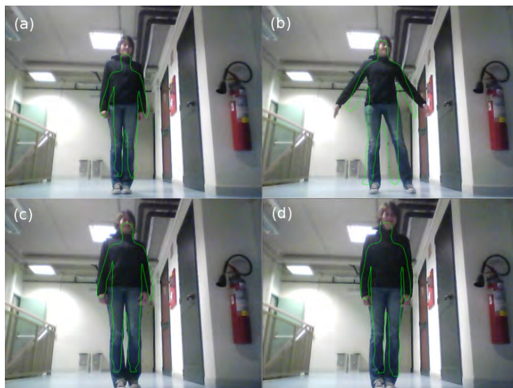
FIGURE 3.7: Automatic Landmarking. Special pose case with a subject approximating to the webcam.
