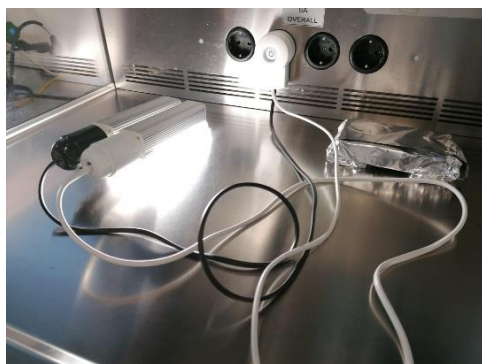
Figure 4.41. Irradiation of a cells plate and the corresponding non-irradiated control covered in aluminium foil under the same conditions.
