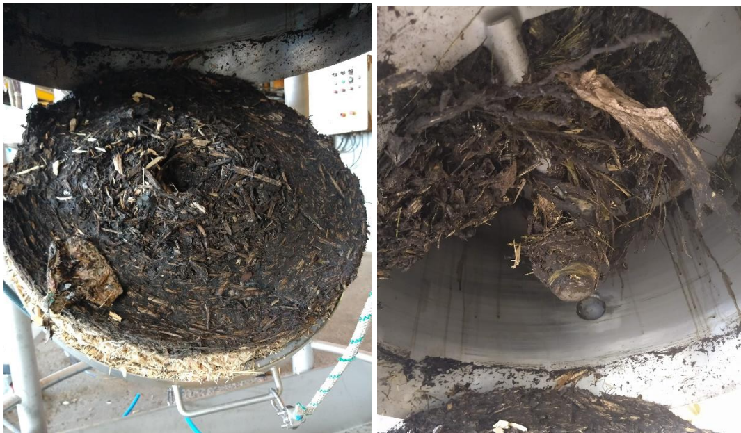
Figure 57: Compacted material at the bottom part and over the stirrer after the composting process.
