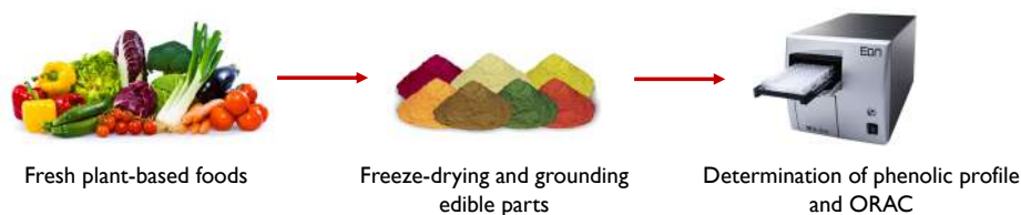
Figure 1. Procedure for the determination of the phenolic profile and antioxidant capacity of plant-based foods.
