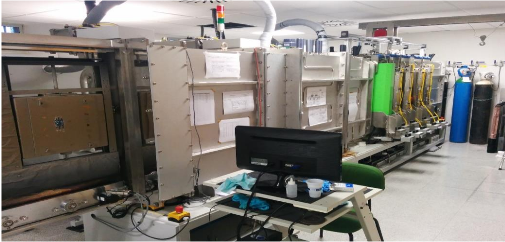
Fig 3. Image of the PVD sputtering system at the university of Zaragoza [2]
