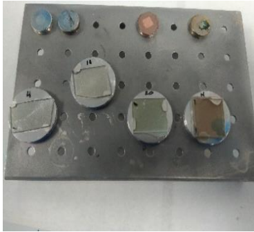
Fig 9.- (Up) Images of the transparent conductive samples analysed on (right) FIB-SEM-EDX instrument.
