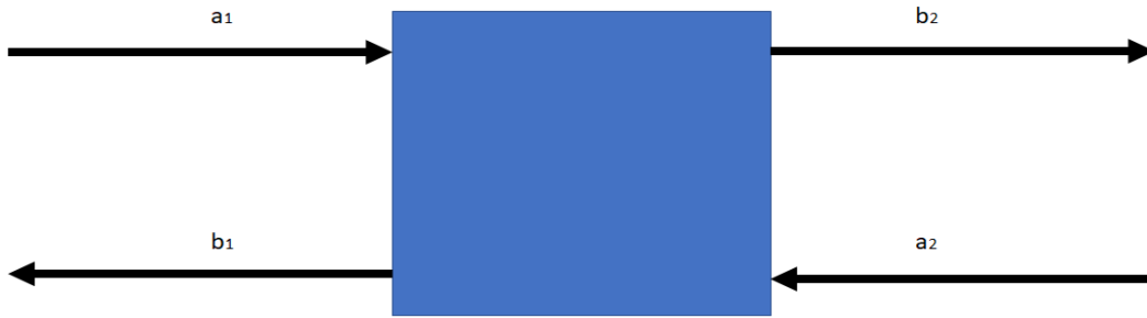
Fig 17. Representation of a two-port network. The blue box represents the system that electromagnetic wave passes through.
