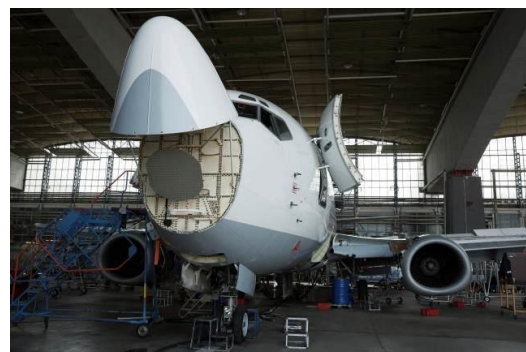
Fig 8 – radar and Radome of a military plane (left) and a comercial plane (right)
