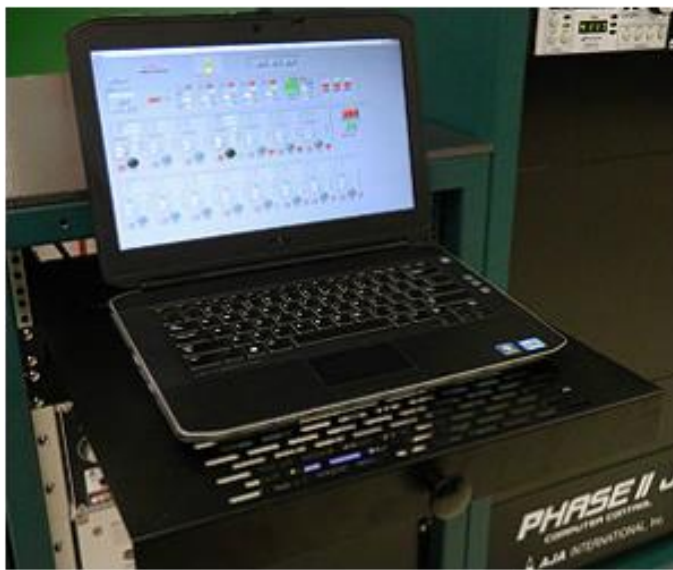
Fig 5 (left). Labview based computer control. Large screen laptop for labview based ATC system computer control.
