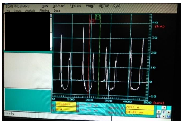
Fig 7 (left) .Image of the Profilometer used at the UB. (down) results of a measurement of a profile of ABC stripes from a etched in a purchased ABC sample.
