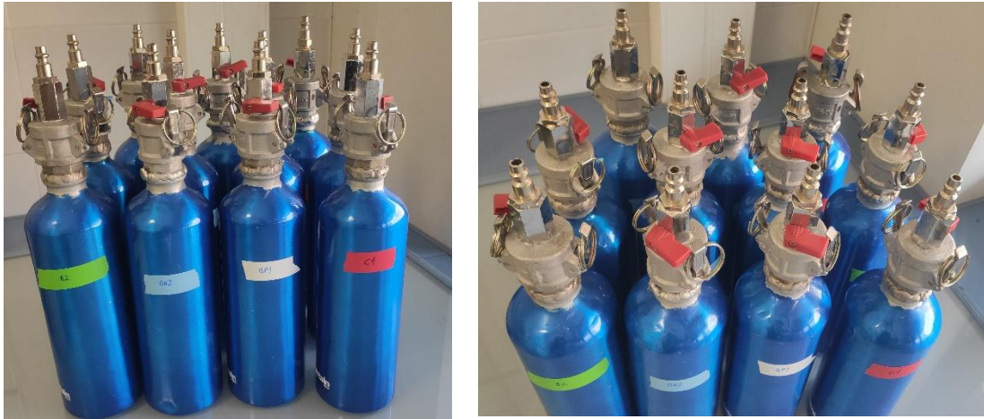
Figure 3.2 Aluminium bottles used in BMP tests.
