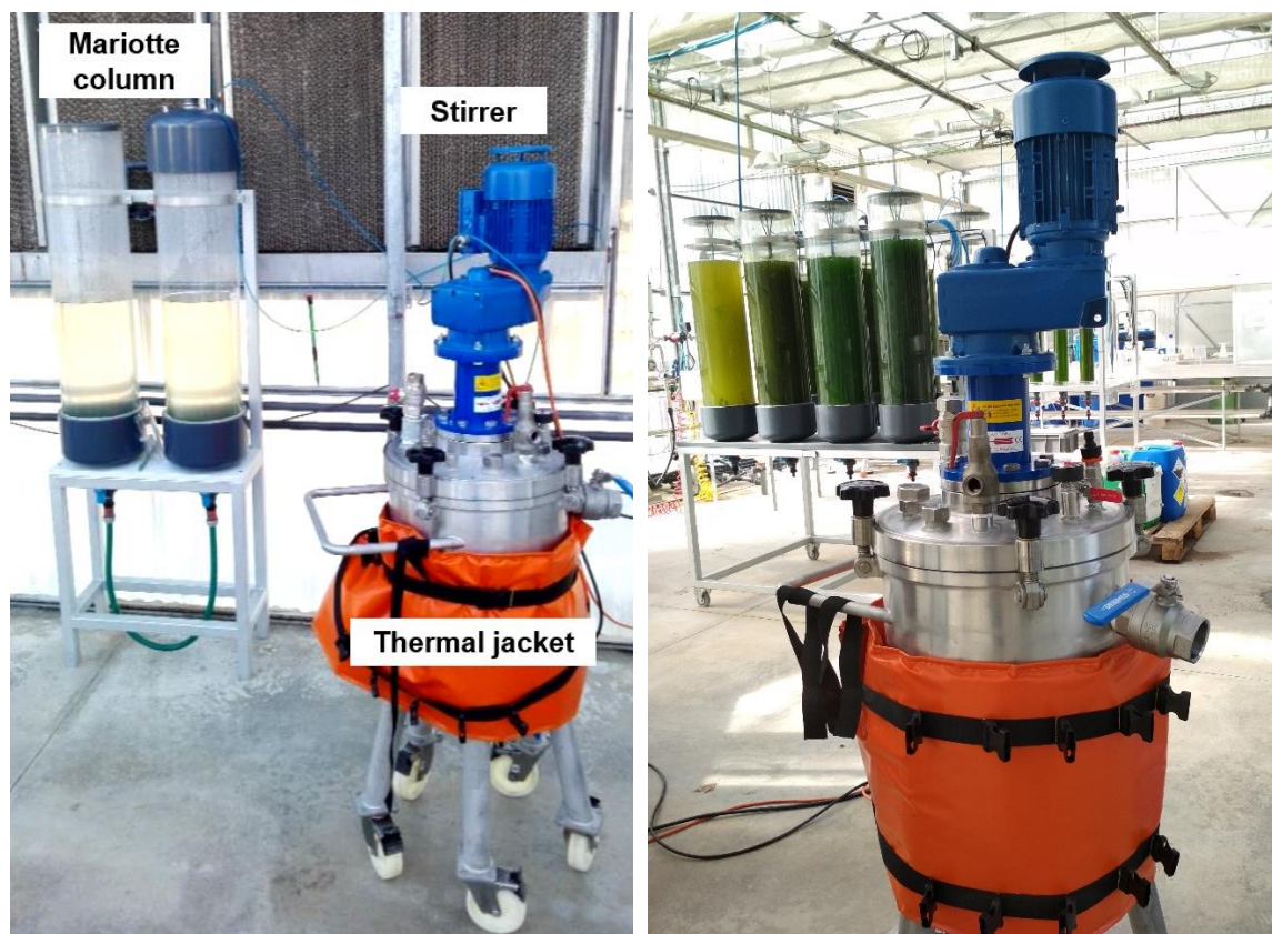
Figure 7.2 Pilot anaerobic reactor.
