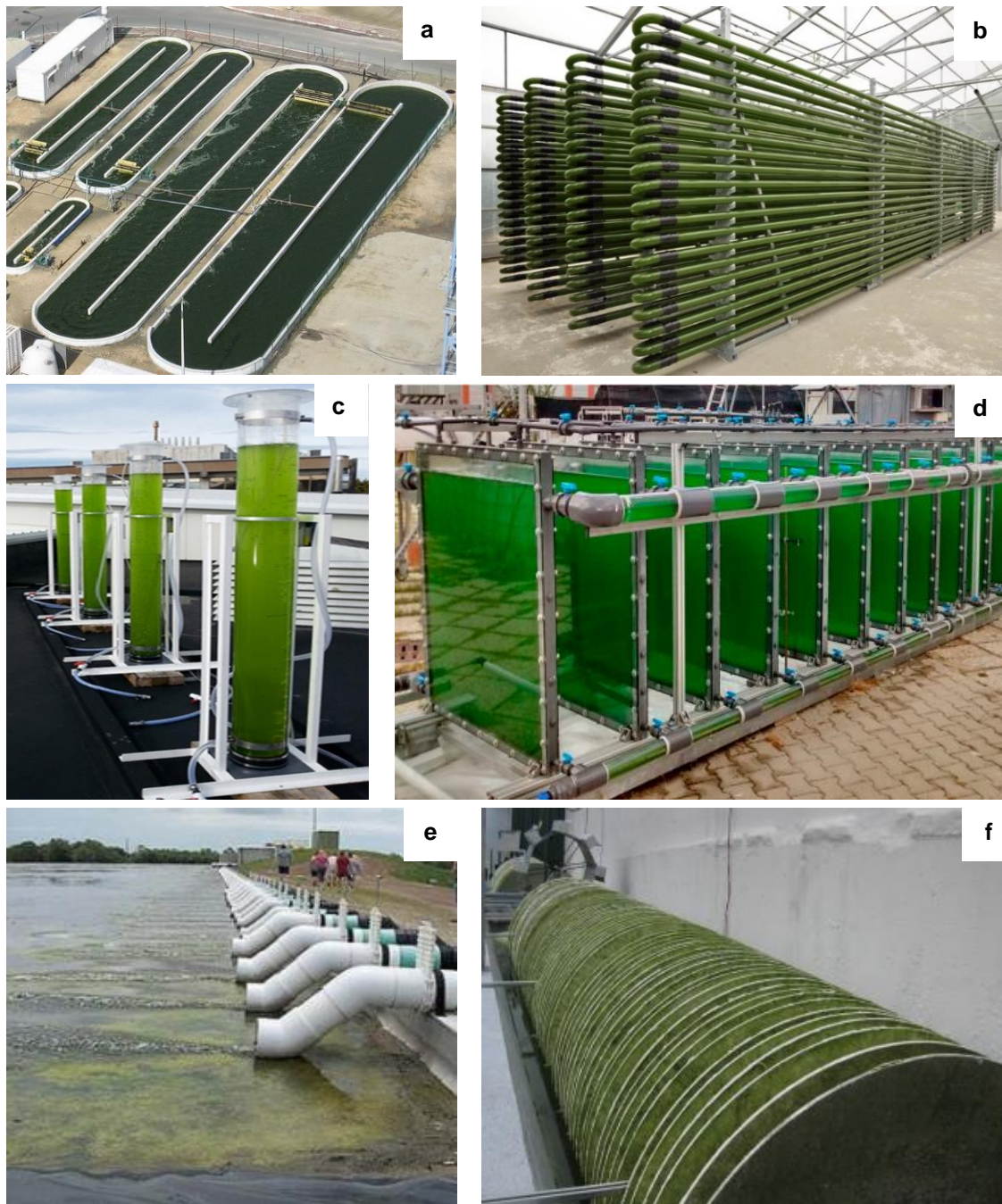
Figure 1.2 Microalgae cultivation systems: (a) HRAP (Yen et al., 2019), (b) tubular PBR, (c) column PBR (Plouviez et al., 2017), (d) flat-plate PBR (Lindblad et al., 2019), (e) algae turf scrubber (U.S. Department of Energy, 2016), and (f) rotating algal PBR (Fernández et al., 2014).
