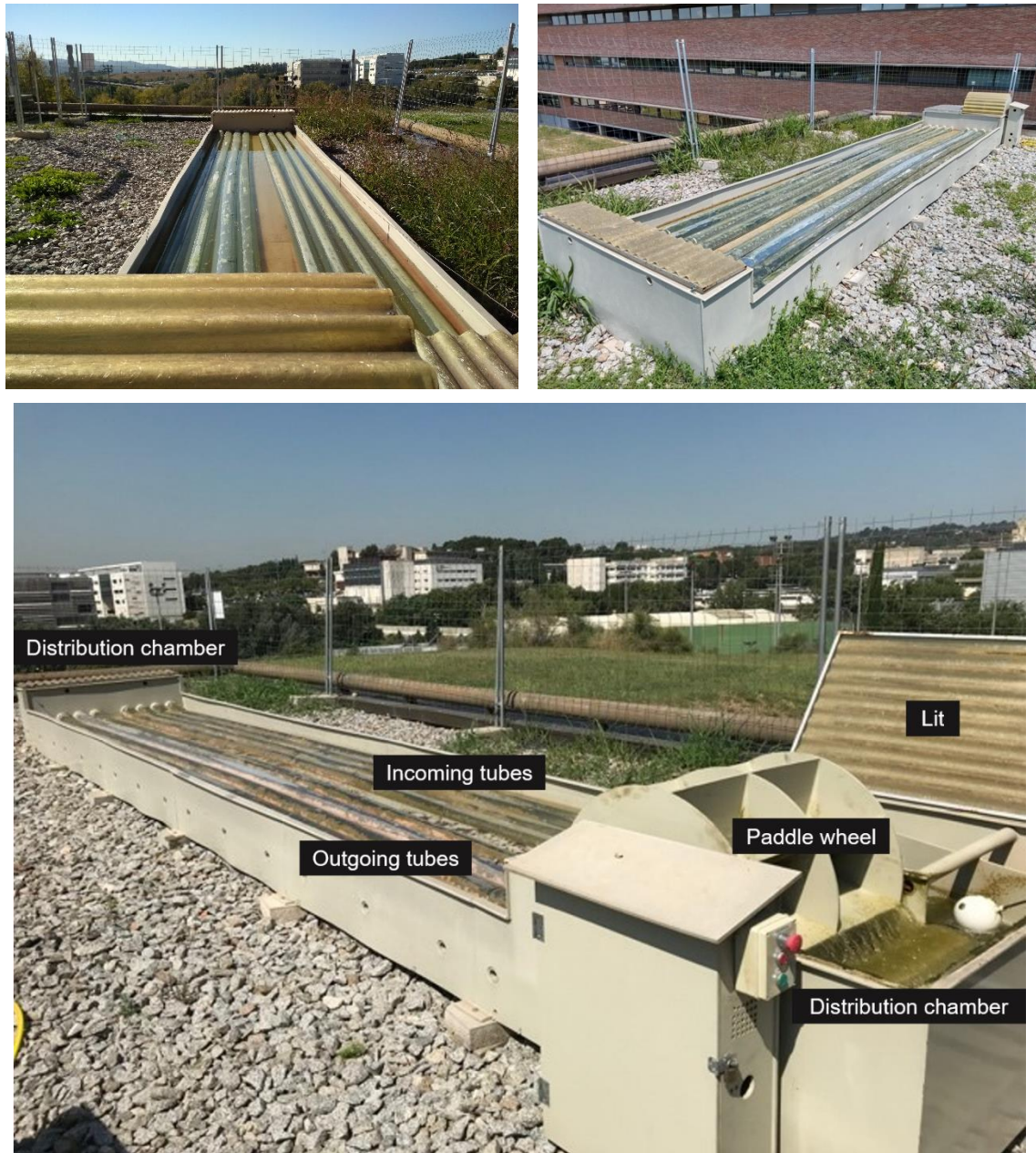
Figure 3.1 Semi-open tubular photobioreactor located at the roof of the Chemical, Biological and Environmental Engineering Department from Universitat Autònoma de Barcelona, Spain.
