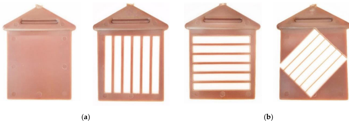
Figure 4. (a) Square sample with dimension 70 × 70 × 1.5 mm, and (b) Square samples from which oriented specimens are laser cut, (from left to right) parallel (0°), perpendicular (90°) and 45° oriented cut.
