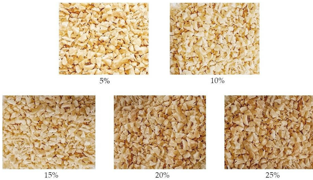
Figure 6. Cellulose pulp composite pellets indicating their respective cellulose composition prepared from Gelimat mixer and later pelletized prior to injection.
