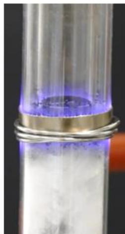
Figure 2.1. a) General DBD plasma-catalytic setup: (1) DBD-catalytic reactor (2) Water condenser (3) Flowmeter (4) Temperature control and measurement (5) Oscilloscope and PC (6) Power supply (7) High voltage probe (8) Current probe. b) DBD-catalytic reactor. c) Plasma and catalyst bed.
