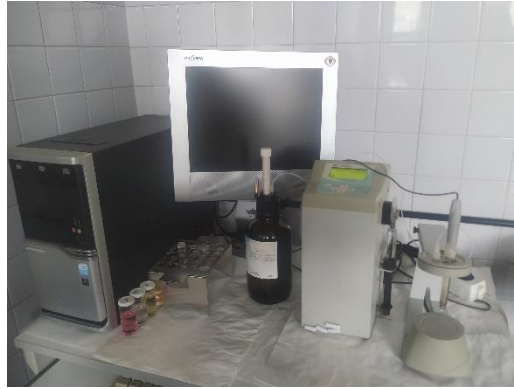
Figure 3.8. Automatic titration device used to measure alkalinity.
