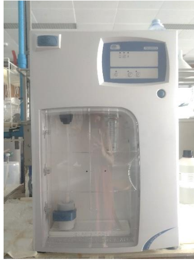
Figure 3.11. Distiller used for the TKN analysis.
