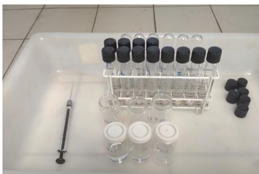
Figure 3.18. Samples preparation before introducing in a digester for 5h.
