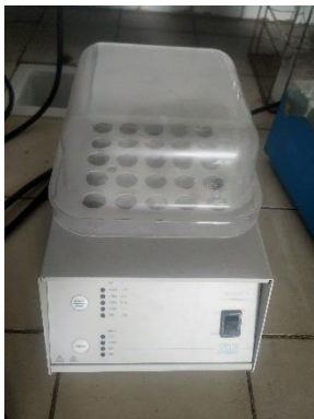
Figure 3.7. Equipments used to carry out COD analysis: COD digester(A) and spectrophotometer (B).
