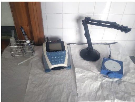
Figure 3.9. Ammonia electrode used to analyse TAN.
