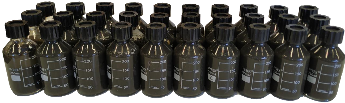
Figure 3.1. Pyrex serum bottles used in batch tests.
