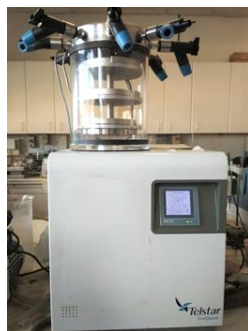
Figure 3.17. Lyophiliser (A) and lyophilised biomass for 24h (B).
