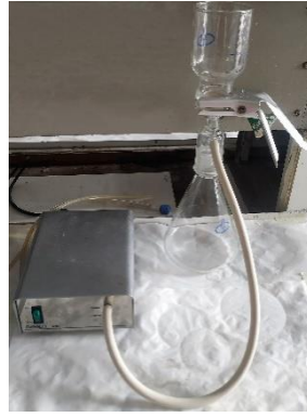
Figure 3.6. Filtration system connected to a vacuum pump.
