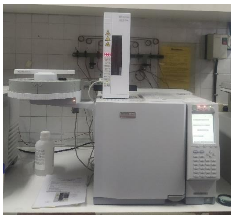
Figure 3.14. Gas chromatograph GC 2010 plus, Shimadzu for VFAs analysis.
