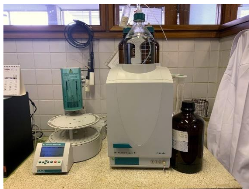
Figure 3.12. Ionic chromatograph with autosampler.
