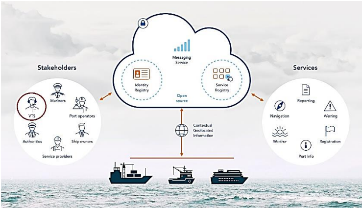
Figure 42. MCP Components for setting up a platform for the provision of maritime services in the context of e-Navigation
