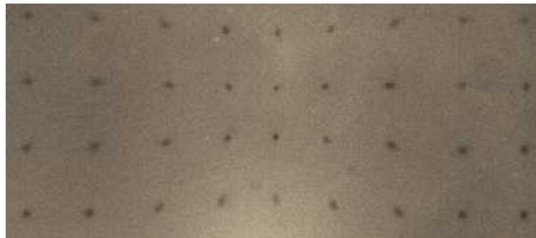
Figure 10.3: A typical picture recorded in Optical Deflectometry measurements. The image of a regular array of black dots (grid spacing d = 5.0 mm) is distorted by the interface deformation.
