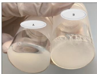
Fig. 4. Visual evaluation of PLGA NPs (A); reconstituted sample of PLGA NPs with 3% maltitol (w/v) (B).
