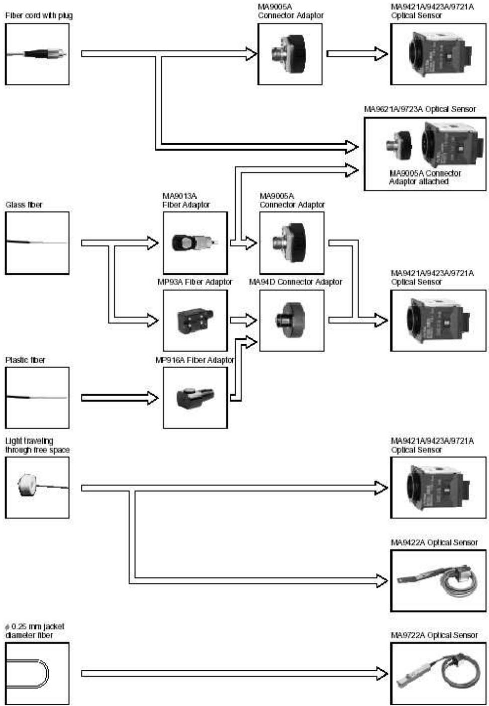
**OPTICAL MEASURING INSTRUMENTS**
