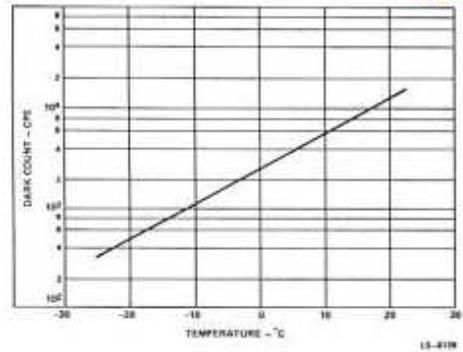
Figure 11. Typical Dark Count vs. Temperature at 5% Photon (830 nm) Deflection Efficiency
