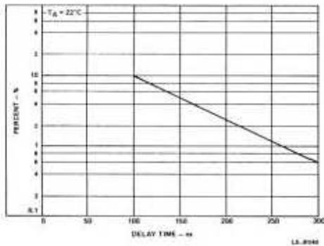
Figure 12. Change of an After-Pulse within the Next 100 ns vs. Delay Time in an Actively Quenched Circuit. (Typical for C30902S, C30921S at  $V_{RR} + 25$ )
