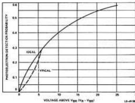
Figure 8. Geiger Mode, Photodetector Detection Probability vs. Voltage Above  $V_{BR}$  ( $V > V_{BR}$ )
