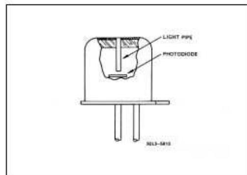
Figure 14. Cutaway of the C30921E, C30921S
