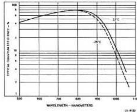
Figure 2. Typical Quantum Efficiency vs. Wavelength
