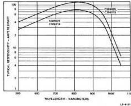
Figure 1. Typical Spectral Responsivity at 22°C
