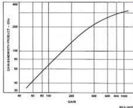
Figure 5. Typical Gain-Bandwidth Product vs. Gain
