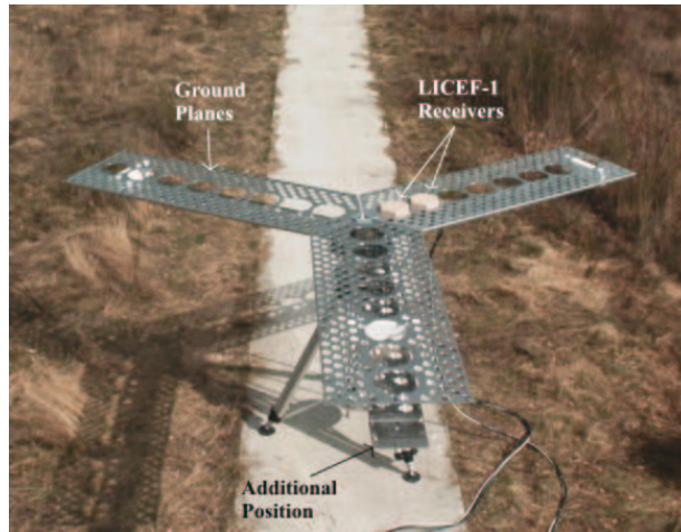
Figure 4.5: Image validation test 3B setup, MIRAS prototype with 9 elements per arm
