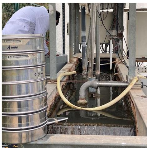
Figure 8 Stainless-steel sieves for filtration of drinking water treatment plant influent
