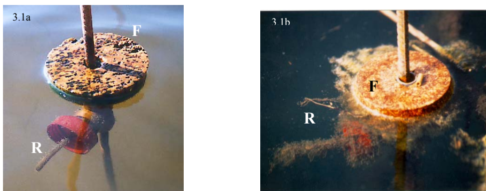
Fig. 3.1a-b Artificial substrata (after one month of exposure) used for sampling periphytic diatoms. R : glass rod used as artificial substratum. F : mobile float.
