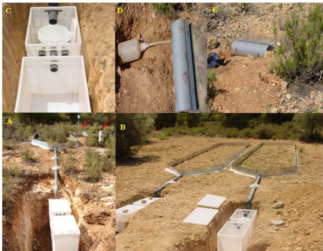
Figure 2.4. Recording rain instrument in the experimental area and closed water erosion plots in the forest (A) and olive grove (B), deposits (C), and sediment traps connected to a plastic bottle (D and E).
