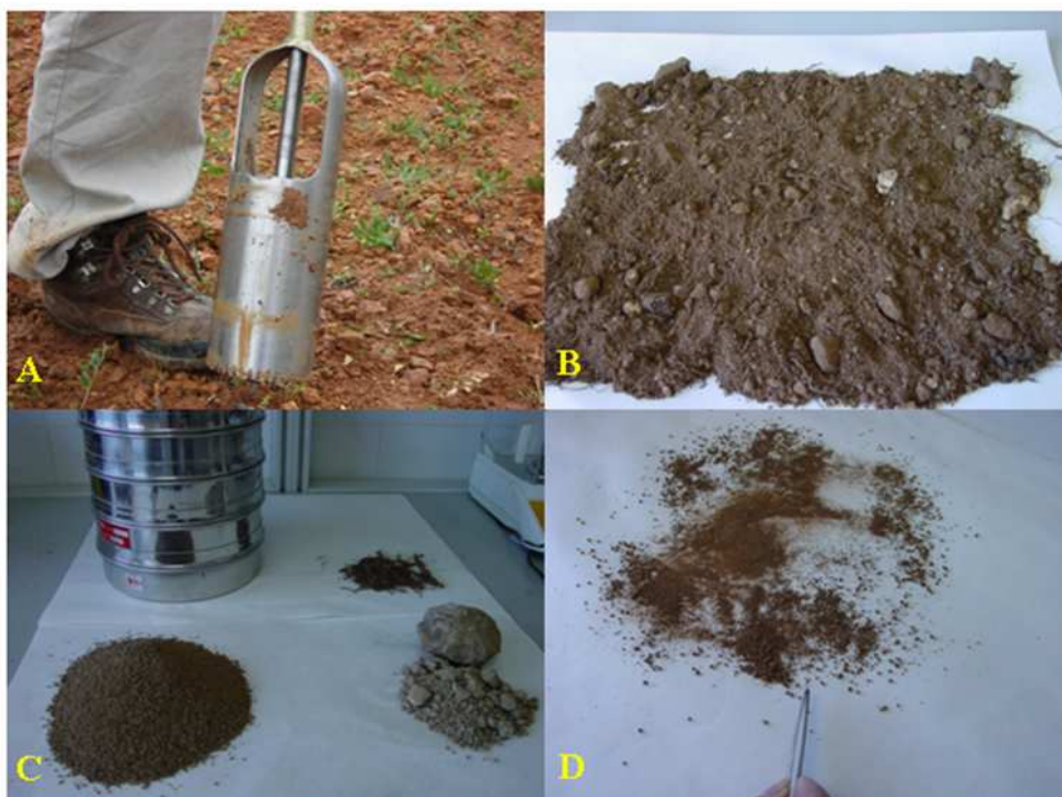
Figure 2.2. Sampling auger (A) and soil from an individual core before being processed for root biomass estimates (B). Soil was rinsed through a series of sieves (C) while roots were hand-picked (D) and placed in a tray.
