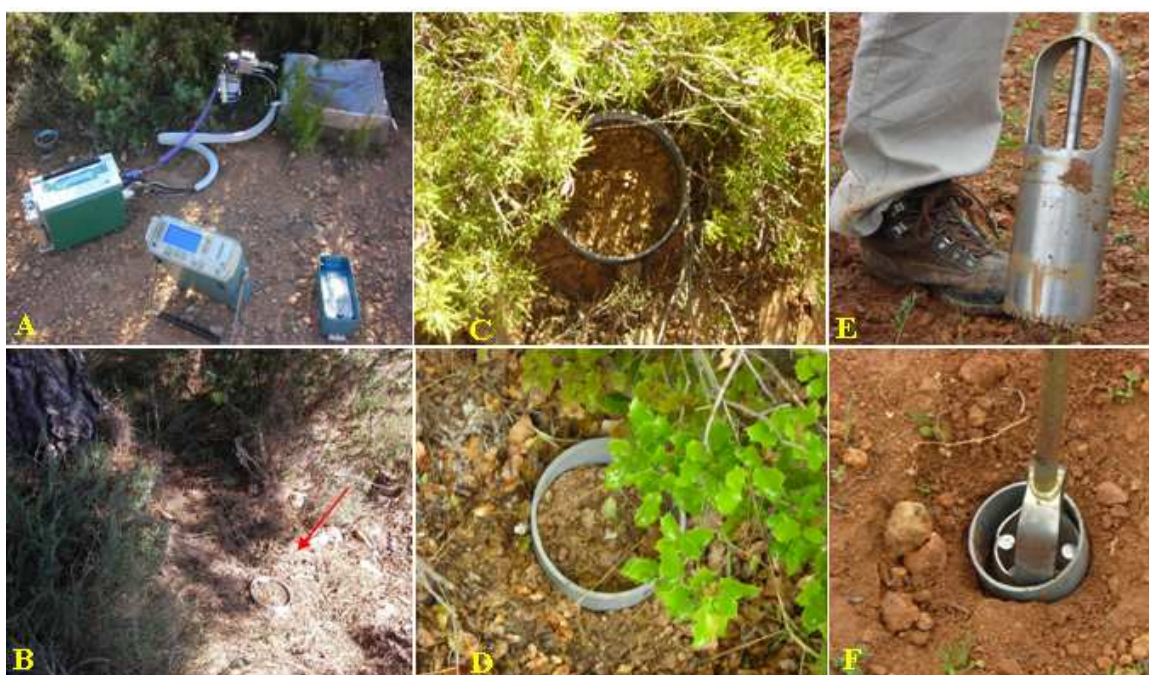
Figure 4.2. Soil respiration chamber, soil temperature probe and TDR (A), soil respiration collars beneath Aleppo pine (B), rosemary (C) and kermes-oak (D), and sampling auger (E) for plant roots and soil sampling (F).
