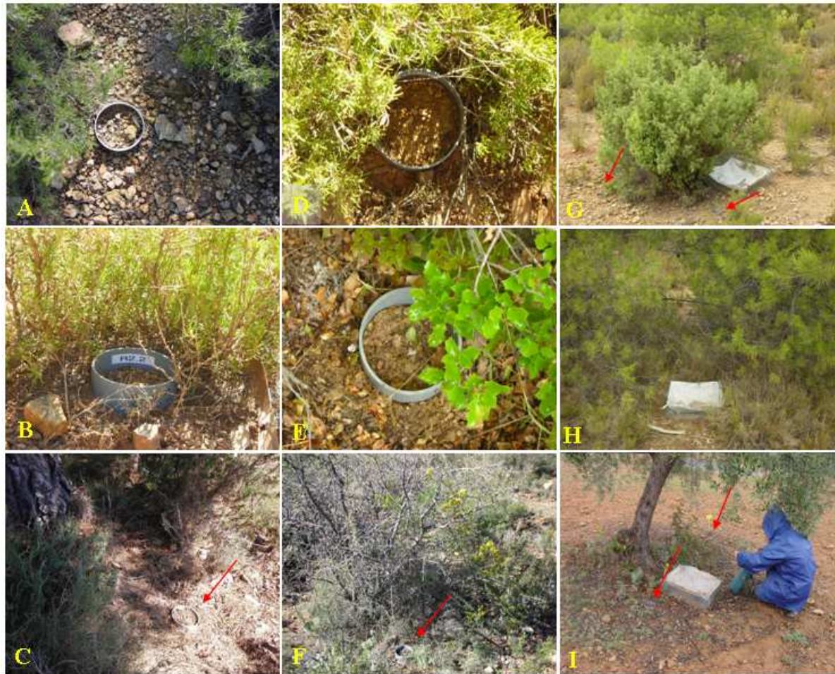
Figure 2.3. Soil respiration collars and/or litter traps beneath the most frequent plant cover types at each site: bare soil (A), Rosmarinus officinalis (B and D), Pinus halepensis (C and H), Quercus coccifera (E), Rhamnus lycioides (F), Juniperus oxycedrus (G), and Olea europaea (I).
