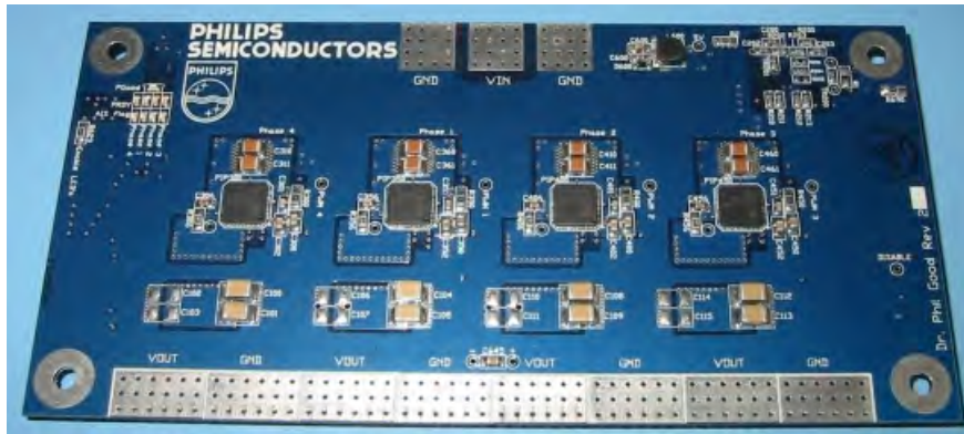
Figure G.3.1 Multiphase voltage regulator test board. Designed by Dr. Phil Good, from Philips Semiconductors.
