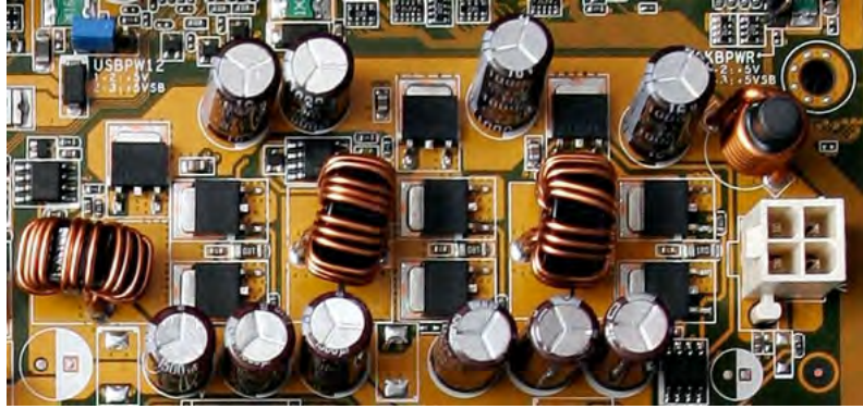
Figure 1.2.15 Three phases low switching frequency VRD of Asus A8N-VM CSM motherboard for AMD's Athlon™ 64bits processors.
