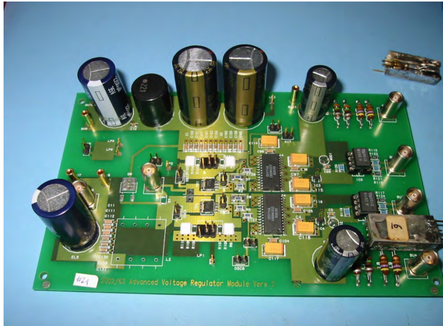
Figure G.1.1 Synchronous buck converter prototype board. Designed by Dr. Tobias Tolle from Philips Research.
