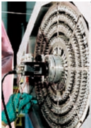
(a) Tuning a the \gamma -ray lens at the CESR.
