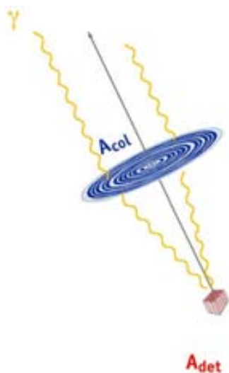
Figure 2.17: The principle of a focusing system for high energy photons. Gamma-rays are concentrated in a focal point behind the collecting area where a small detector is located (figure from von Ballmoos (2005)).
