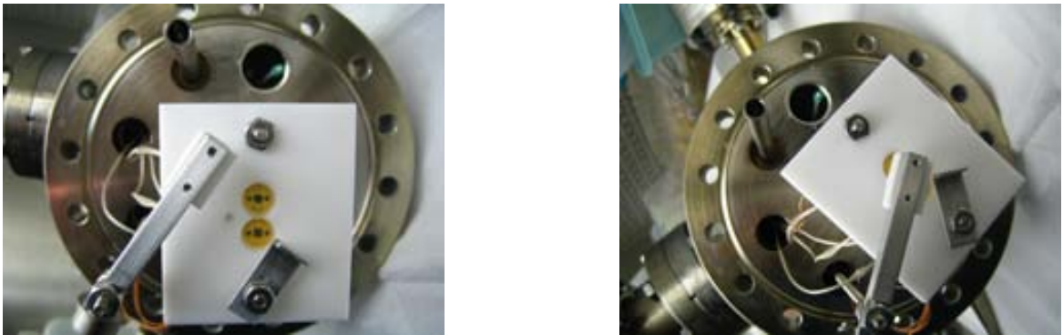
Figure 6.10: Photography of SiPMs detectors with the source device placed in front of the detector(right) and outside the detector(left).
