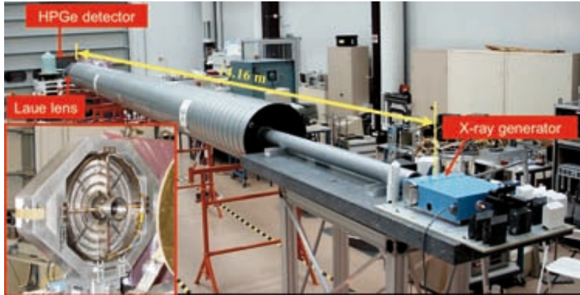
Figure 3.6: Optical bench for tuning the Laue lens at the CESR (Toulouse).
