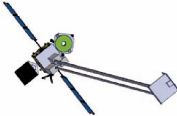
Figure 2.19: A possible design for a space-borne \gamma -ray telescope base on Laue lens (figure from DUAL collaboration)
