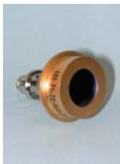
Figure 6.20: Picture of the 16mm diameter windowless LAAPD (SD 630-70-75-500) from Advanced Photonix, Inc.
