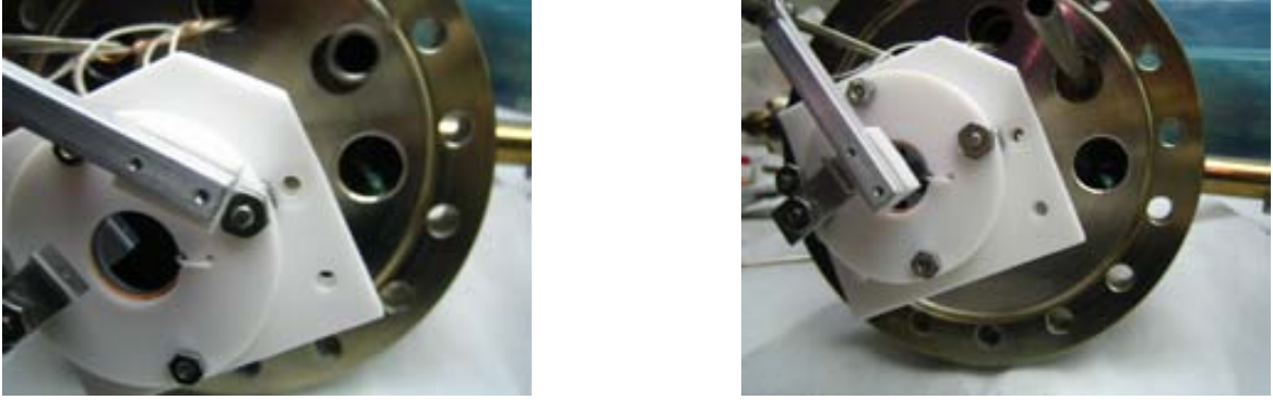
Figure 6.21: Picture of the LAAPD mounted on a PTFE disk with the alfa source device placed in front of the detector (right) and outside the detector (left).
