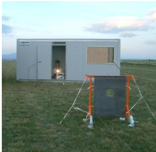
Figure 3.13: Photograph of the lead diaphragm (front) and the X-ray tube (back) used in the test.
