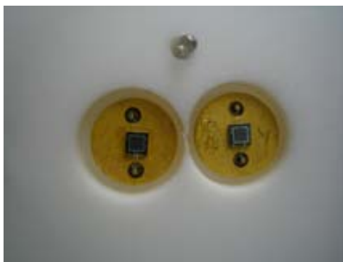
Figure 6.9: Photo of two SiPMs mounted side by side on a PTFE Teflon plate. The platinum resistor (RTD) to measure the temperature of the Teflon plate is also shown on top.
