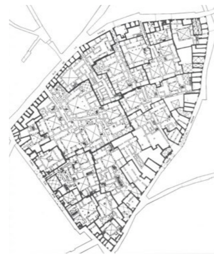
Figure I.8: Tunis Medina - Urban fabric with superimposed house plans: deep territorial structure as a consequence of successive included territories. (cfr. fig. 8.4: N.J. Habraken, "The Structure of the Ordinary" MIT Press Cambridge 1998, p147)
