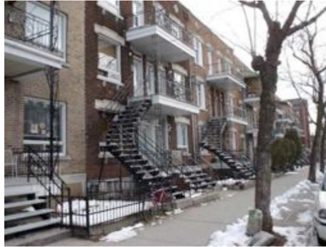
Figure I.37: residential neighbourhood in Montreal (Canada): seeking shorter linear sequences with no shared spaces (shared entrance hall), avoiding integration values by adding external staircases to a multi-family housing project. (image from www.bricoleurbanism.org )
