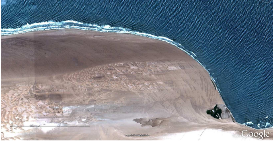
Figure 1.5: Wave refraction around a large scale shoreline undulation at Conception Bay in Namibia. Notice the decrease in wave energy in the surfzone at the downdrift flank due to wave energy dispersion. The horizontal line indicates 5 km and the north is in the right of the image (source: Google Earth).
