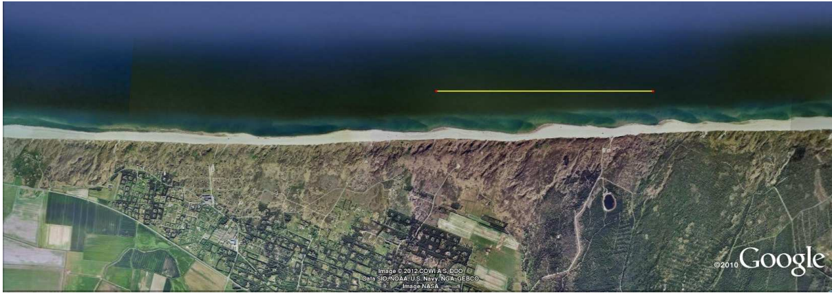
Figure 7.19: Shoreline undulations related to a crescentic bar on the Danish coast, south of the Nissum Fjord. The north is in the right of the image and the horizontal line indicates 2 km (source: Google Earth).
