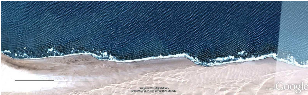
Figure 1.2: Large scale shoreline sand waves on the coast of Namibia in Conception Bay. Notice that the length scale of the undulations is much bigger than the width of the surfzone. The horizontal line indicates 5 km and the north is in the right of the image (source: Google Earth).
