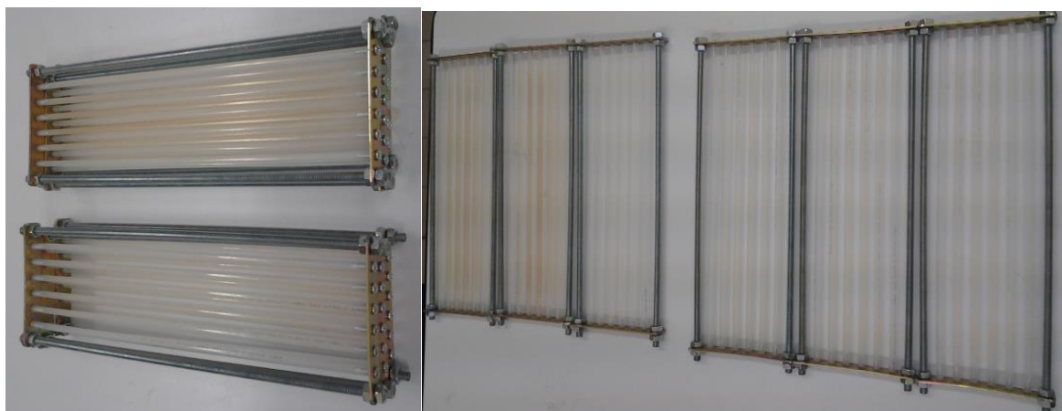
Figure 3.18. Standard and treated PA tubes (left) and standard and treated LDPE tubes (right).
