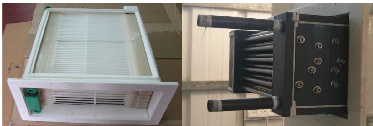
Figure 2.16. Internally water-cooled made of HDPE (left) and titanium (right) [11].
