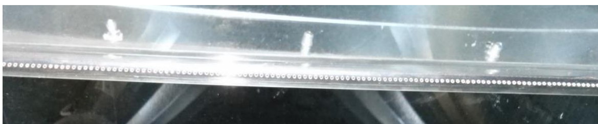
Figure 3.10. Liquid distributor with 1 mm circular holes separated by 2 mm between each one.
