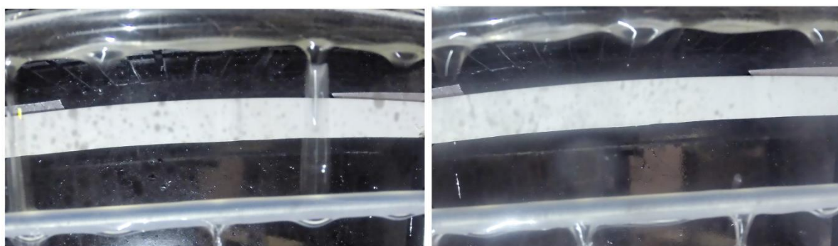
Figure 3.27. Full wetted standard (left) and treated (right) PA tubes at droplet mode.
