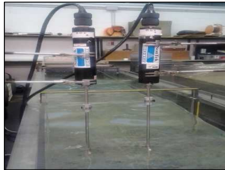
Figure 2.2 Photograph of acoustic doppler velocimeter (16 Mhz- ADV, Sontek Inc.).
